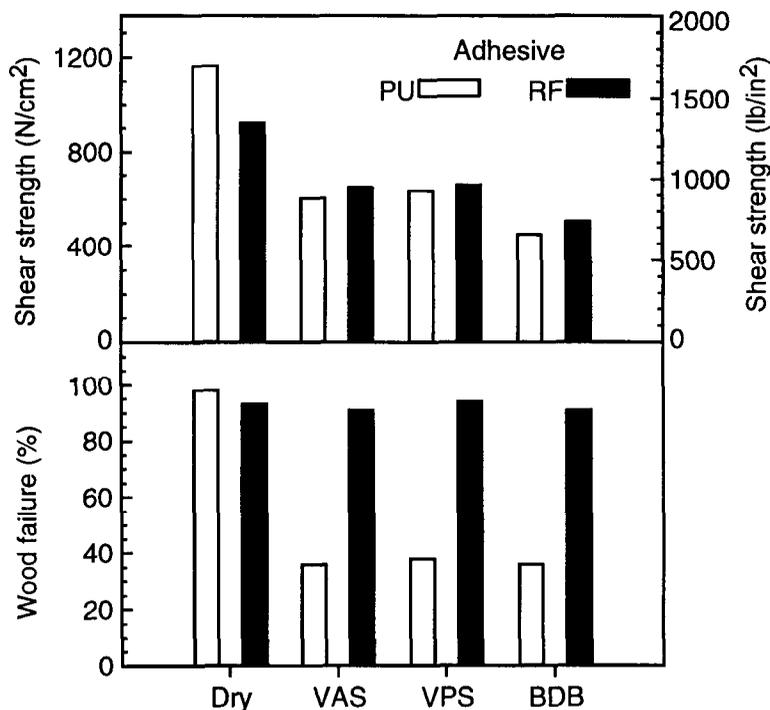
Figure 3. – Shear strength and wood failure of four polyurethane (PU) adhesives (averaged) compared with a resorcinol (RF) adhesive on Douglas-fir after one dry and three wet tests (VAS = vacuum-atmospheric pressure water soak; VPS = vacuum-pressure water soak; BDB = boil-dry-boil).
