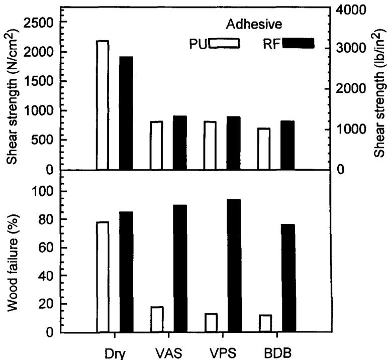
Figure 2. – Shear strength and wood failure of four polyurethane (PU) adhesives (averaged) compared with a resorcinol (RF) adhesive on yellow birch after one dry and three wet tests (VAS = vacuum-atmospheric pressure water soak; VPS = vacuum-pressure water soak; BDB = boil-dry-boil).
