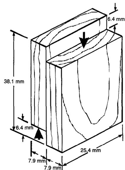
Figure 1. – Modified compression-loaded block-shear specimen with 6.5-cm<sup>2</sup> (1.0-in.<sup>2</sup>) shear area (1 mm = 0.04 in.).
