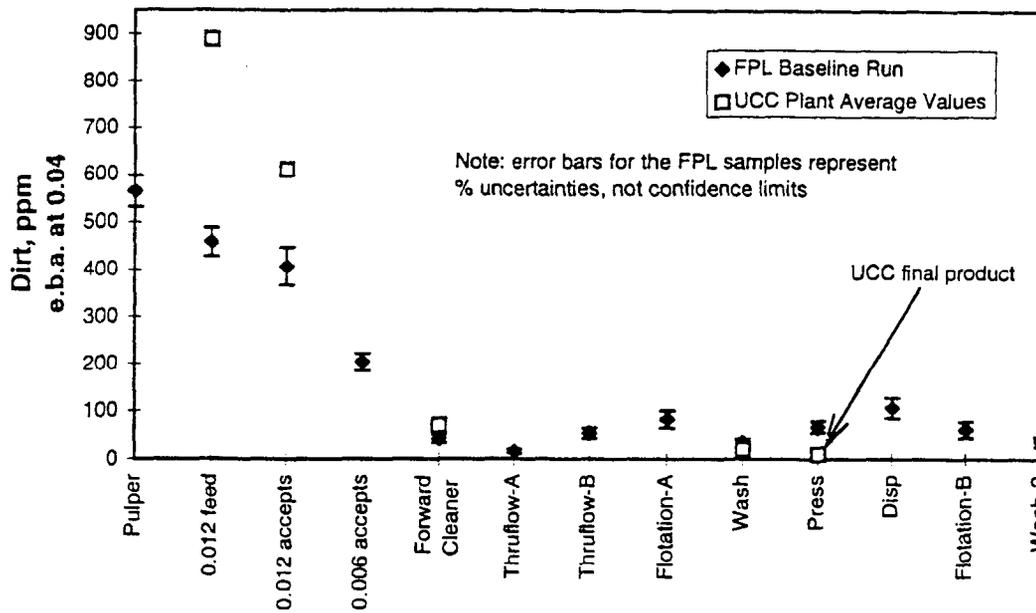
Figure 7 - FPL Pilot Baseline Run: Dirt Profile as Measured at UCC
