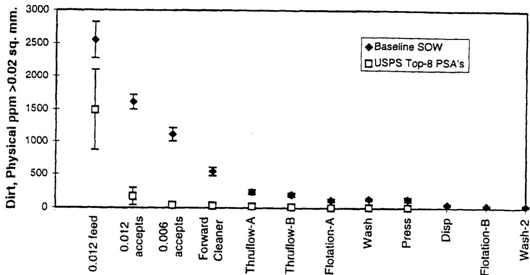
Figure 6 - FPL Pilot Baseline Run: Dirt Profile as Measured at FPL
