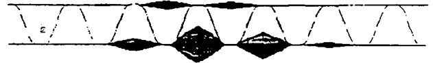
FIGURE 5. Buckled liner for fiberboard 2 (adhesive modulus is 10 times that of liner). Aspect ratio = 1.0; Buckled stress factor = 36.9.
