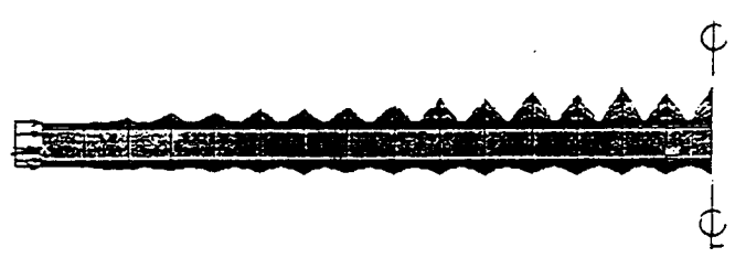
FIGURE 6. Buckled liner for fiberboard 2 (adhesive modulus is 10 times that of liner). Aspect ratio = 3.0; Buckled stress factor = 41.6
