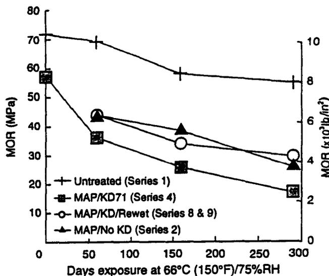
Figure 4. — Effects of FR retention, rewetting, and leaching on bending strength of 1/2-inch (12-mm) plywood.
