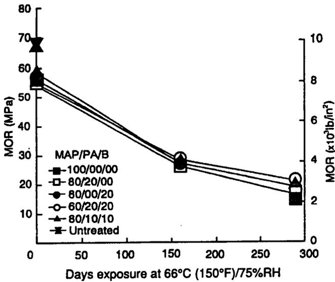
Figure 3. — Effect of various percentages of FR mixtures on bending strength of 5/8-inch (16-mm) plywood. PA = phosphoric acid; B = boric acid.
