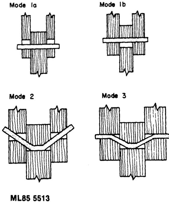
Figure 4.6—Failure modes assumed in the European Yield Model.
