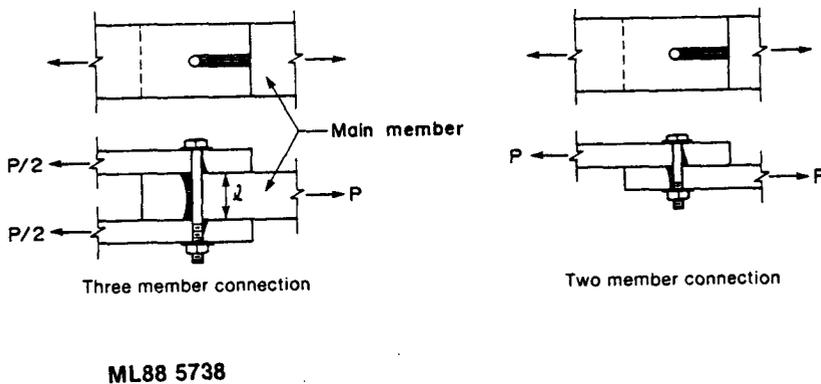
Figure 4.2—Configuration and Stress Distribution for a Laterally Loaded Bolted Connection.
