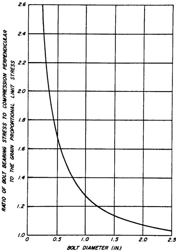
Figure 4.5—Bearing Stress Perpendicular-to-Grain as Affected by Bolt Diameter.
