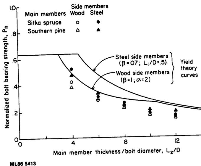
Figure 4.8—Results for Proportional Limit (Trayer 1932) and Yield Load (European Yield Theory) for Three-Member Connections with Steel and Wood Side Plates and Parallel-to-Grain Loading ( $F_y = 45000$  Psi,  $f_c = 5130$  Psi,  $F_{em} = 3280$  Psi).
