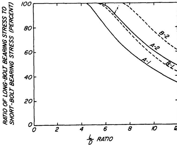
Figure 4.4—Variation in Bolt Bearing Stress at Proportional Limit Perpendicular-to-Grain vs. Slenderness Ratio. Curves A-1 and A-2 are for Experimental Average Compression Perpendicular Stresses of 1140 and 570 Psi, Respectively. Curves B-1 and B-2 Modify Curve A to Establish Design Strengths.
