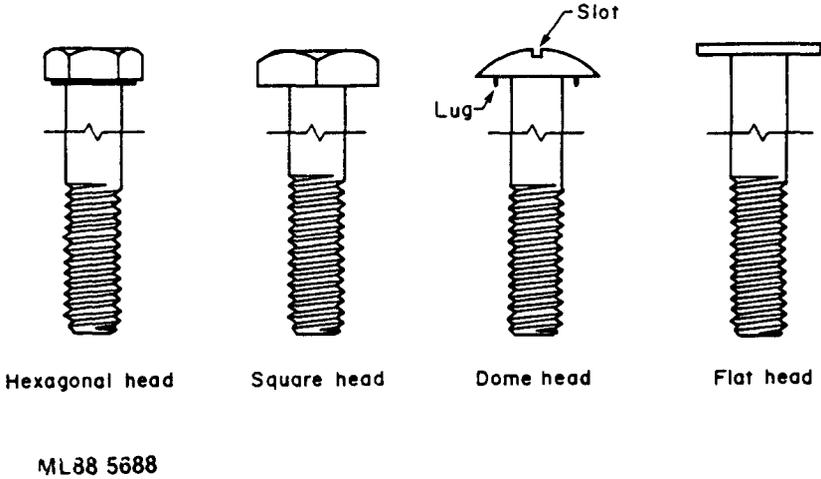
Figure 4.1—Typical Bolt Types.
