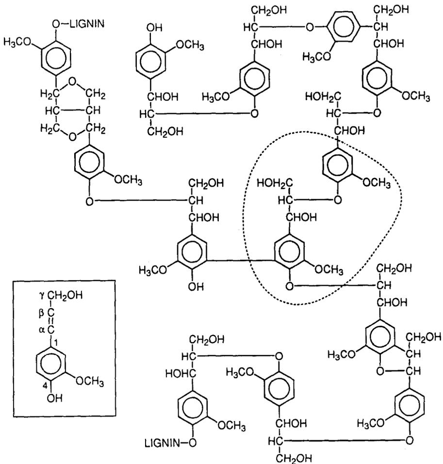
**Fig. 2.1.** Common structures of softwood lignin, with an example of the major arylglycerol- $\beta$ -aryl ether structure circled. The inset shows coniferyl alcohol, the phenylpropanoid building block of softwood lignin.
