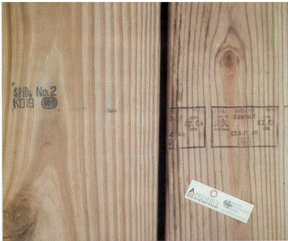
**Look for the mark to be sure what you're getting.** Grade marks, such as the ones on these two pieces of pressure-treated lumber, indicate the maximum moisture content of the wood, which is information that's good to know if you're going to use the wood to build a deck. Some pressure-treated wood will carry two marks, one from the mill and one from the pressure treater.
