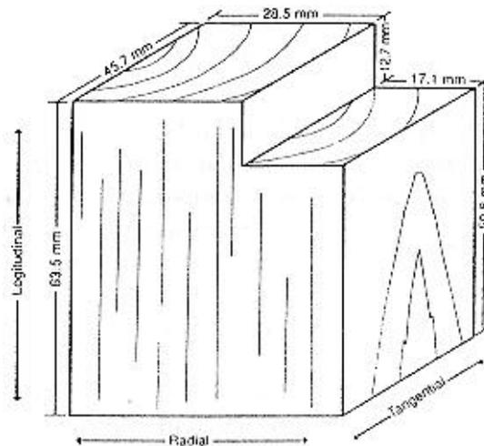
Figure 4. Shear block dimensions
