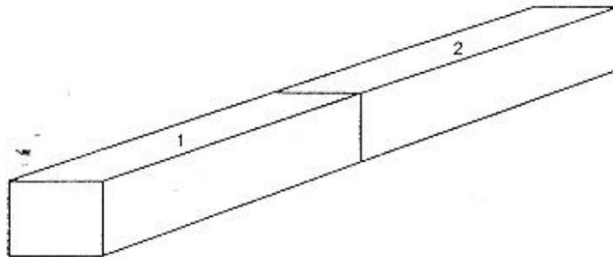
**Figure 3.** Specimen cut from stick obtained from flitches: the half located nearest the ground level was used for static bending test and physical property assessment; the other half was used to obtain all other mechanical properties.
