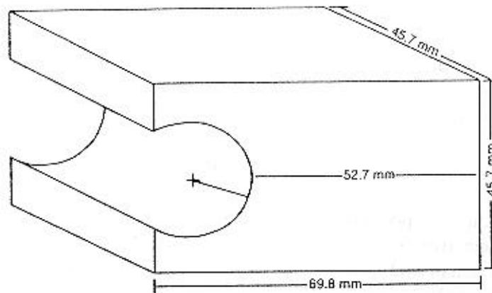
**Figure 5.** Cleavage specimen dimensions. Half the specimens were tested so that crack propagated in the radial plane; the remaining half were tested so that crack propagated in the tangential plane. Radius of notch was 12.5 mm.
