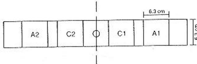
**Figure 2.** Specimen cutting scheme showing end view of a pith-centred flitch
