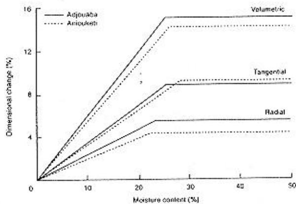
Figure 6. Dimension changes used to calculate the fibre saturation point for (-) adjouaba and (- - -) aniouketi
