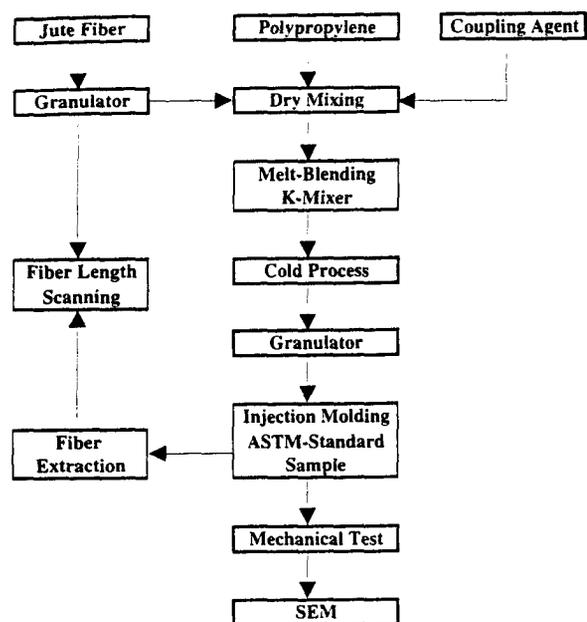
Figure 1 Flow chart of sample production and testing.
