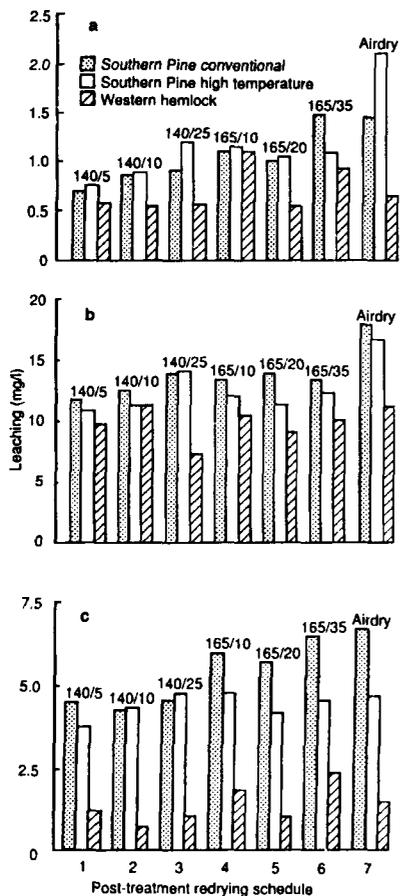
Figure 2. — Total cumulative leaching by redrying schedule (defined as dry-bulb/wet-bulb depression temperatures) and species group: a) chromium; b) arsenic; c) copper.
