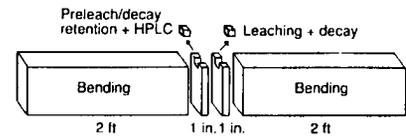
Figure 1.— Diagram of cutting pattern in the 6-foot (1.8-m) boards.
