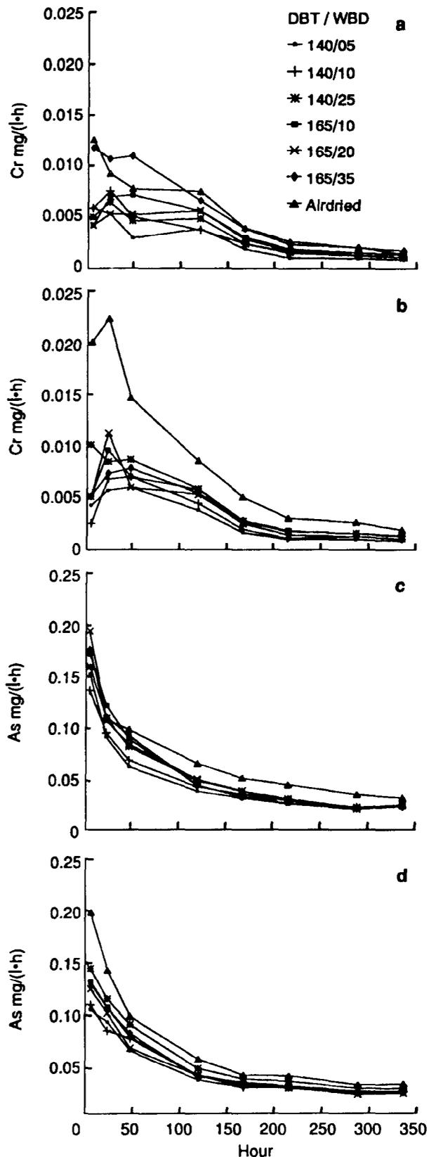
Figure 3. — Rate of leaching by redrying treatment and species group: a) southern pine—conventional kiln dried (chromium); b) southern pine—high-temperature kiln-dried (chromium); c) southern pine—conventional-temperature kiln-dried (arsenic); d) southern pine—high-temperature kiln-dried (arsenic).
