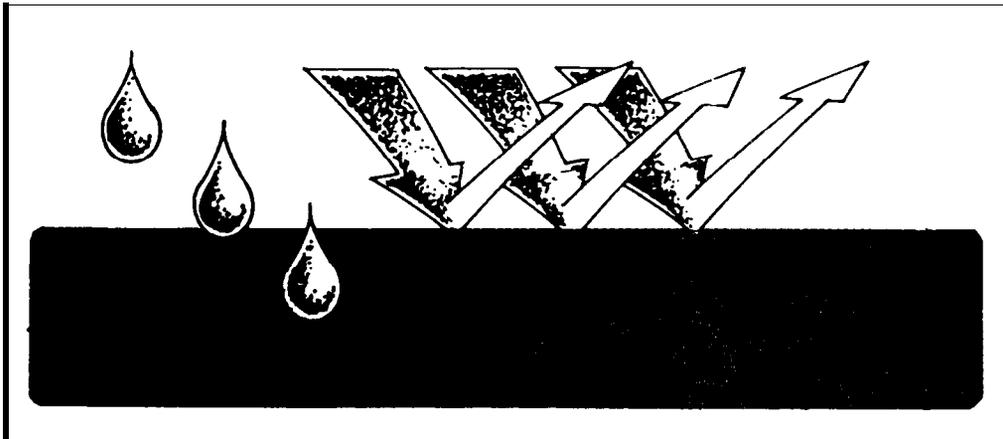
As might be expected, application of a clear or lightly pigmented finish will do little to mask the color or even-out the appearance. In light colored coatings the CCA green will appear to "bleed-through" the finish. This is not a physical bleeding of the treatment but, rather, an optical show-through effect. The use of darker colors, more opaque finishes and/or a second coat can reduce or eliminate the green show-through and even-out the substrate appearance.
