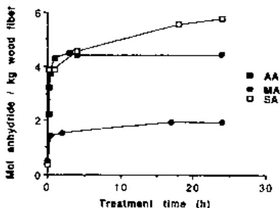
FIG. 2. Molar gains of aspen fiber esterified with acetic (AA), maleic (MA), and succinic (SA) anhydrides.
