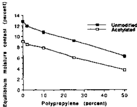
FIG. 7. Equilibrium moisture content of unmodified or acetylated aspen fiber compared to polypropylene content.
