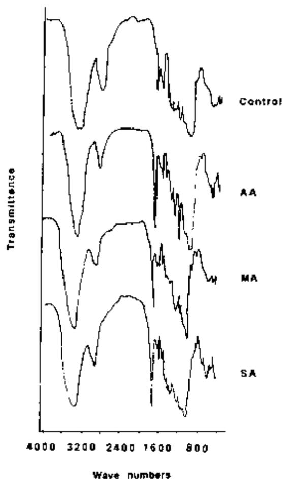
FIG. 3. FTIR spectra for control and esterified aspen fiber. AA is acetic anhydride, MA maleic anhydride, and SA succinic anhydride.
