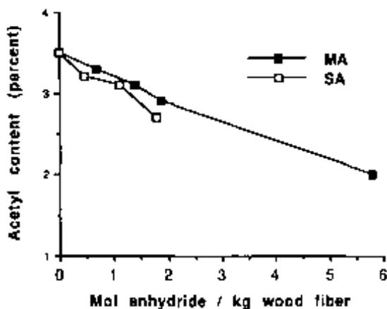
FIG. 4. Transesterification of hemicellulosic acetyl groups by maleic (MA) and succinic (SA) anhydrides.
