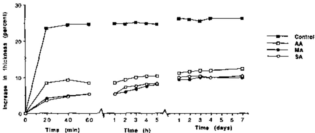
FIG. 8. Swelling history (water-soaked specimens) of control fiberboards and fiberboards modified with acetic (AA), maleic (MA), or succinic (SA) anhydrides and 5% phenol-formaldehyde resin.
