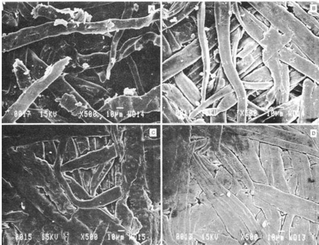
FIG. 14. Scanning electron micrographs of control and modified fiberboards. A, Control. B-D, Fiberboards modified with different anhydrides (weight Percent gain in parentheses): B, acetic (20%); C, maleic (20%); and D, succinic (58%).
