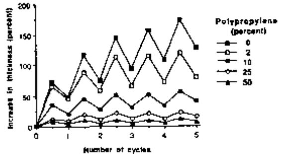
FIG. 13. Increase in thickness during cyclic water-swelling test of fiberboards made with acetylated aspen fiber and various amounts of polypropylene.
