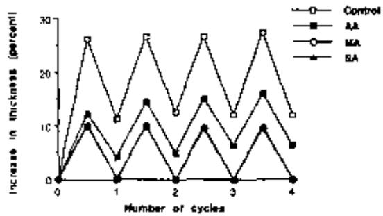
FIG. 9. Increase in thickness during cyclic water-swelling tests of control fiberboards and fiberboards modified with acetic (AA), maleic (MA), and succinic (SA) anhydrides and 5% phenol-formaldehyde resin.
