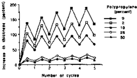
FIG. 12. Increase in thickness during cyclic water-swelling test of fiberboards made with unmodified aspen fiber and various amounts of polypropylene.
