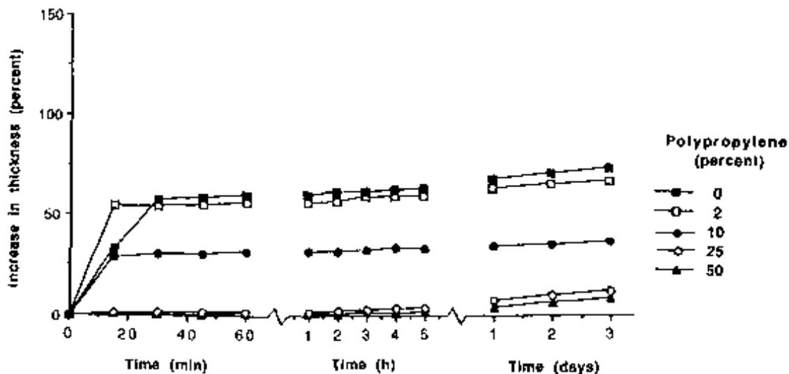
FIG. 11. Swelling history (water-soaked specimens) of fiberboards made with acetylated aspen fiber and various amounts of polypropylene.
