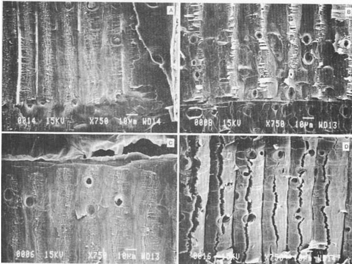
FIG. 5. Scanning electron micrographs of southern yellow pine blocks. A, Control. B-D, Blocks modified with different anhydrides (weight percent gain in parentheses): B, acetic (22%); C, maleic (4.5%); and D, succinic (61%).
