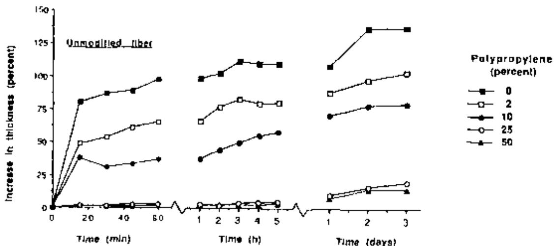
FIG. 10. Swelling history (water-soaked specimens) of fiberboards made with unmodified aspen fiber and various amounts of polypropylene.
