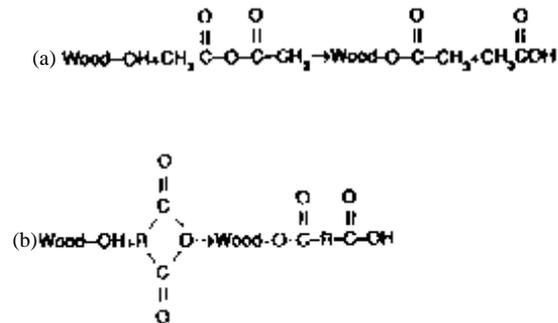
FIG. 1. Esterification reactions for aspen fiber reacted with (a) acetic anhydride or (b) maleic anhydride (when R is  $-\text{HC}=\text{CH}-$ ) or succinic anhydride (when R is  $-\text{CH}_2-\text{CH}_2-$ ).
