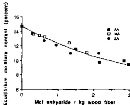
FIG. 6. Equilibrium moisture content of aspen fiber esterified by reaction with acetic (AA), maleic (MA), and succinic(SA) anhydrides.
