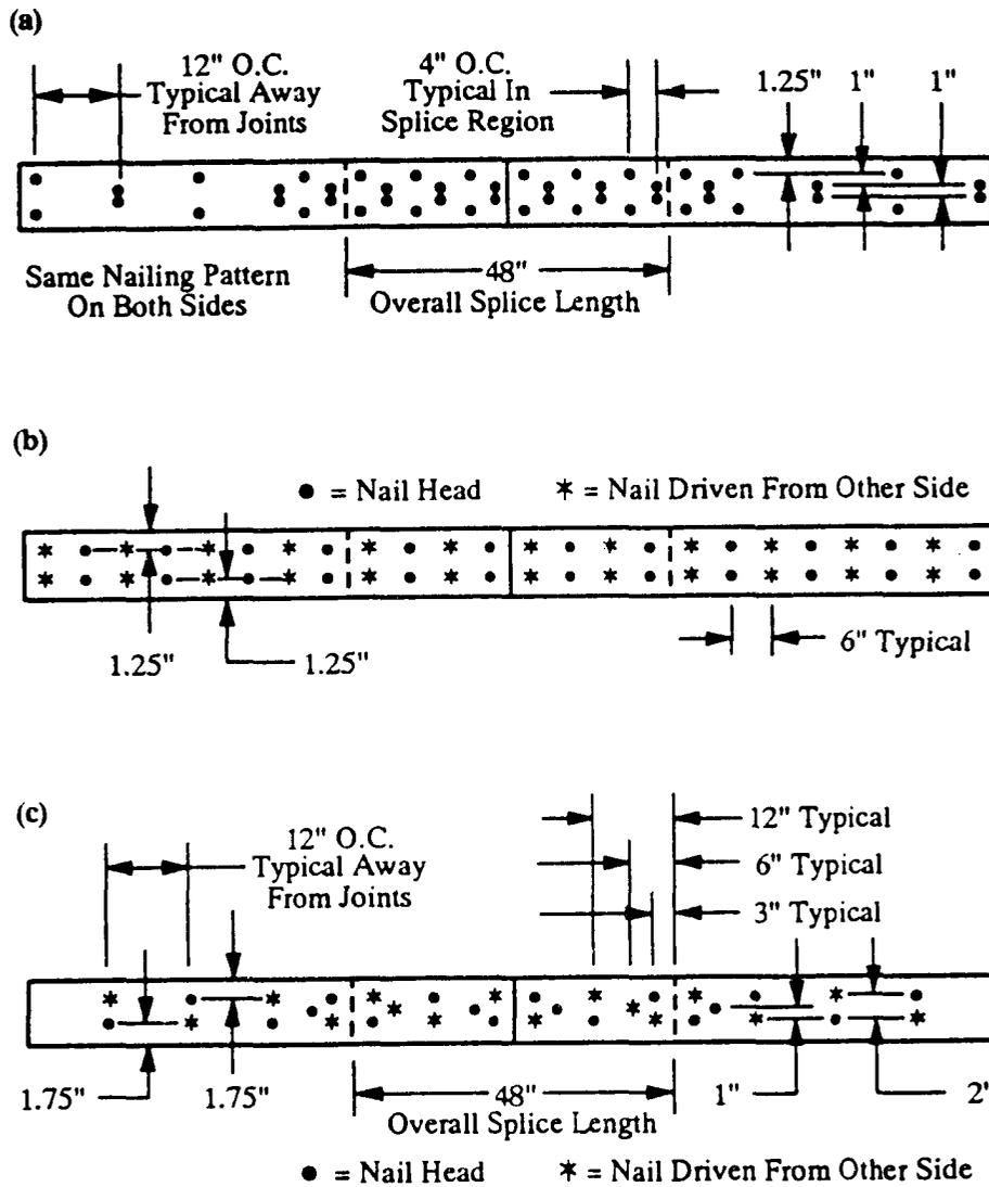
Figure 7.8—Nailing patterns for three-layer, nail-laminated posts with staggered butt joints. Nailing patterns used by (a) Woeste<sup>32</sup> (similar to pattern used by DeBonis et al.<sup>20</sup> and Woeste et al.<sup>33</sup>), (b) Winistorfer et al.<sup>30</sup> (not recommended for use), and (c) Bohnhoff et al.<sup>15</sup>.
