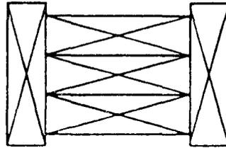
**Figure 7.7—Cover plates used to increase the bending capacity of a laminated post about axis H-H.**
