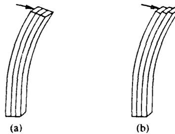
**Figure 7.3—(a) Interlayer rigidity of a horizontally glued laminated post, (b) interlayer slip of a horizontally mechanically laminated post.**
