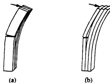
**Figure 7.4--(a) Interlayer slip in the joint region of a vertically mechanically-laminated post, (b) delamination in the joint region of a horizontally nail-laminated post.**
