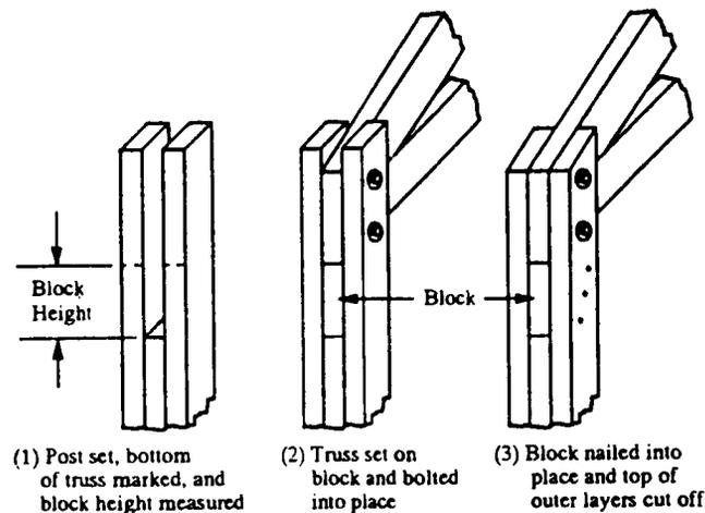
**Figure 7.2—Placement of a truss between the outer layers of a three-layer assembly.**
