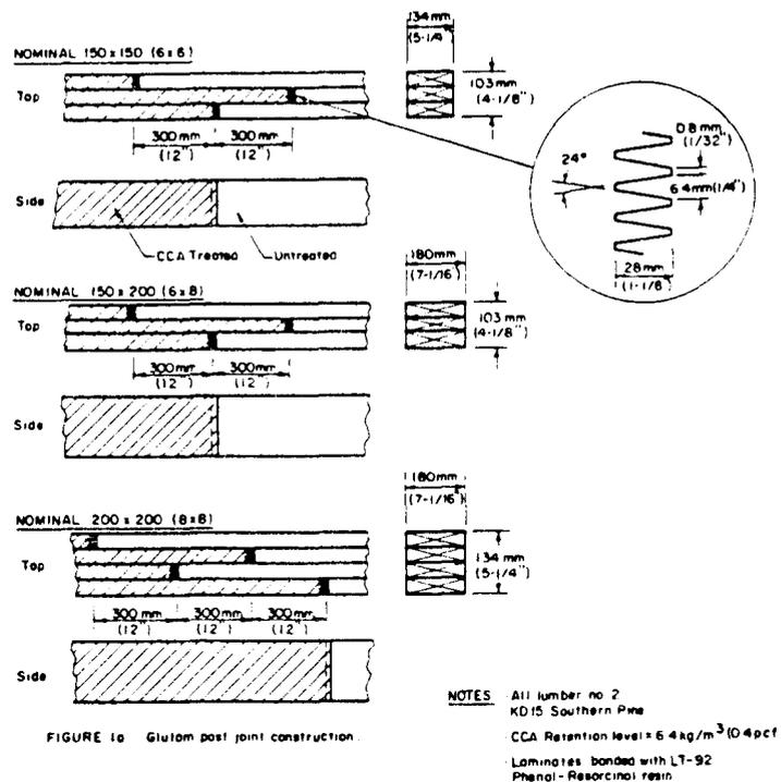
**Figure 7.6—Glued-laminated posts tested by Wright et al.<sup>36</sup> in compression and in bending about axis V-V.**
