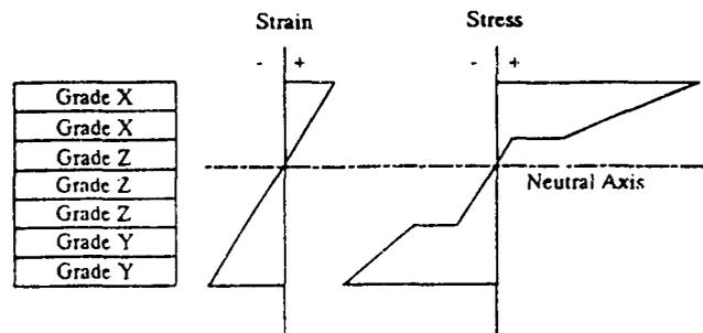
**Figure 7.5—Strain and corresponding stresses in horizontally glued laminated assembly manufactured from differential lumber grades.**
