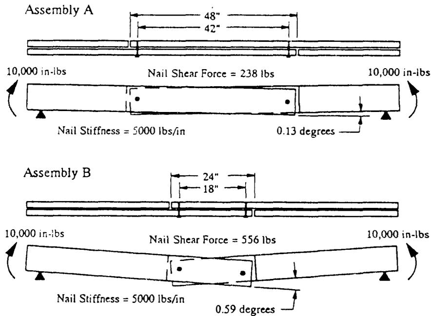
**Figure 7.12—Influence of splice length on nail shear force and stiffness of a two-layer assembly.**
