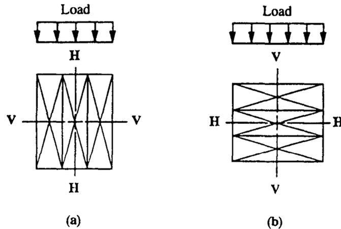
Figure 7.1—(a) Vertically laminated, (b) horizontally laminated posts.
