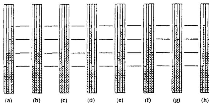
**Figure 7.14—Arrangement of joints in four-layer assemblies, fixed spacing of end joints.**
