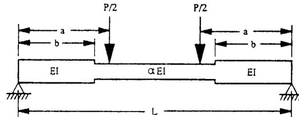
**Figure 7.11—Model of a spliced assembly under a two-point loading; reduced flexural rigidity in the spliced region.**
