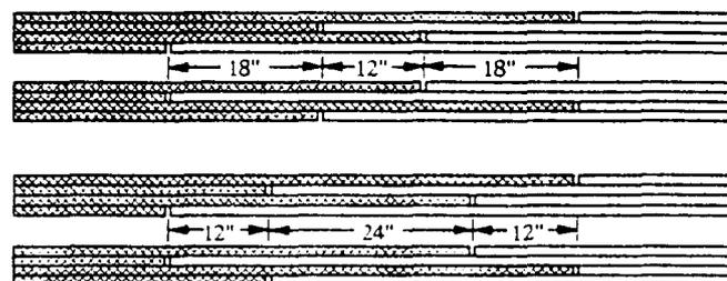
**Figure 7.15—Arrangement of joint in four-layer assemblies, spacing of end joints not fixed.**
