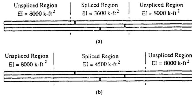
**Figure 7.10—Effect of selection of spliced region length on effective flexural rigidity.**
