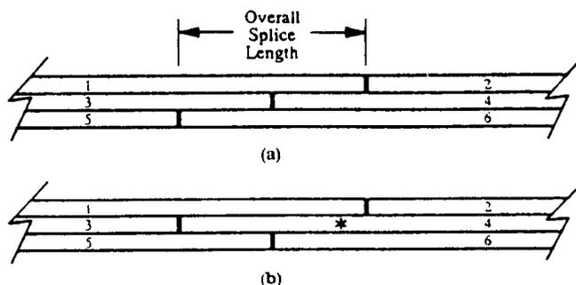
**Figure 7.13—Arrangement of joints in spliced nail-laminated posts: (a) step pattern, (b) commonly used stagger pattern, \* point of high stress.**
