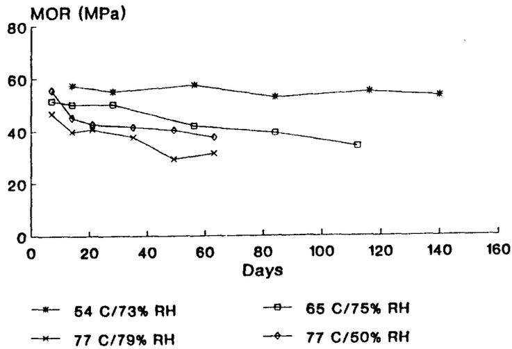
Figure 3 Effect of exposure to various temperatures on modulus of rupture (MOR) of monoammonium phosphate-treated plywood.
