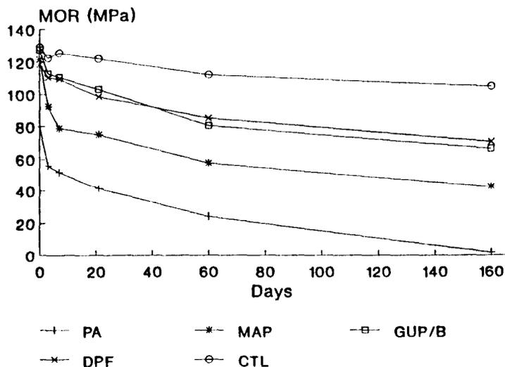
Figure 1 Effects of four fire retardants on bending strength of 16- by 35- by 305-mm clearwood specimens exposed to steady-state exposure at 82°C (180°F) and 50% RH (CTL = untreated; PA = phosphoric acid; MAP = monoammonium phosphate; GUP = guanylurea phosphate; DPF = dicyandiamide-phosphoric acid-formaldehyde).
