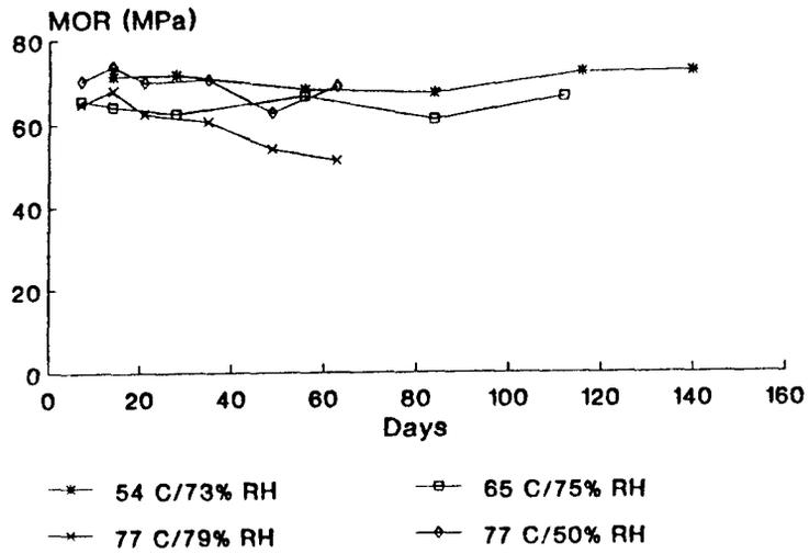
Figure 2 Effect of exposure to various temperatures on modulus of rupture (MOR) of untreated plywood.
