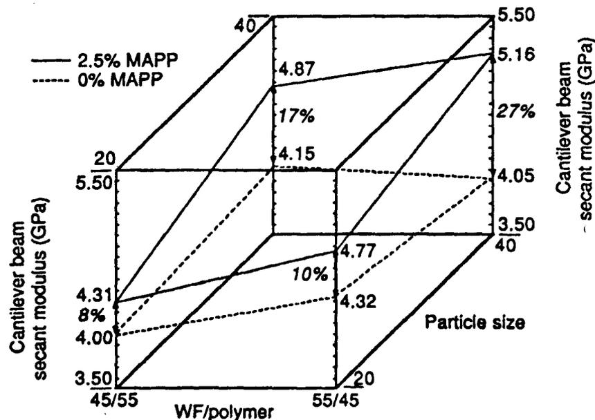
Figure 2. — Cantilever beam secant (9°) modulus of extruded composite as a function of wood flour to total polymer weight ratio, wood flour particle size, and MAPP-1 level. (All data points are the average of results for one and three extrusions. MAPP levels are weight percentages of total system.)
