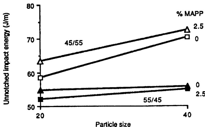
Figure 4. — Unnotched impact energy of extruded composite as a function of wood flour particle size, wood flour to total polymer weight ratio, and MAPP level.
