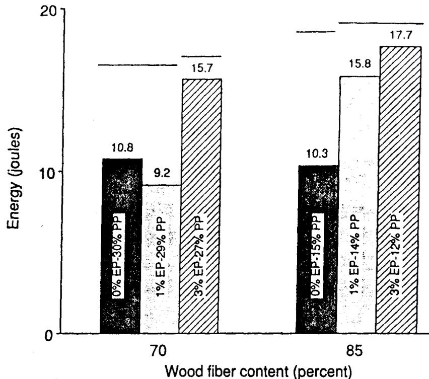
Figure 7. — Impact energy of nonwoven web composite as a function of wood fiber content and MAPP-2 level. (EP is MAPP-2; PP is polypropylene; percentages are weight percent of total system. Bars connected by a solid line are not significantly different at the 95% confidence level.)
