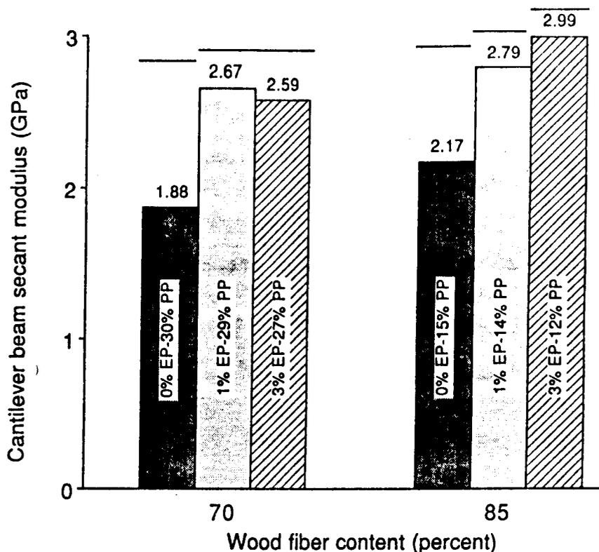
Figure 9.— Cantilever beam secant ( $9^\circ$ ) modulus of nonwoven web composite as a function of wood fiber content and MAPP-2 level. (EP is MAPP-2; PP is polypropylene; percentages are weight percent of total system. Bars connected by a solid line are not significantly different at the 95% confidence level.)
