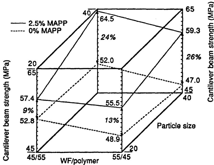
Figure 1. — Maximum cantilever beam strength of extruded composite as a function of wood flour to total polymer weight ratio, wood flour particle size, and MAPP-1 level. (All data points are the average of results for one and three extrusions, MAPP levels are weight percentages of total system.)
