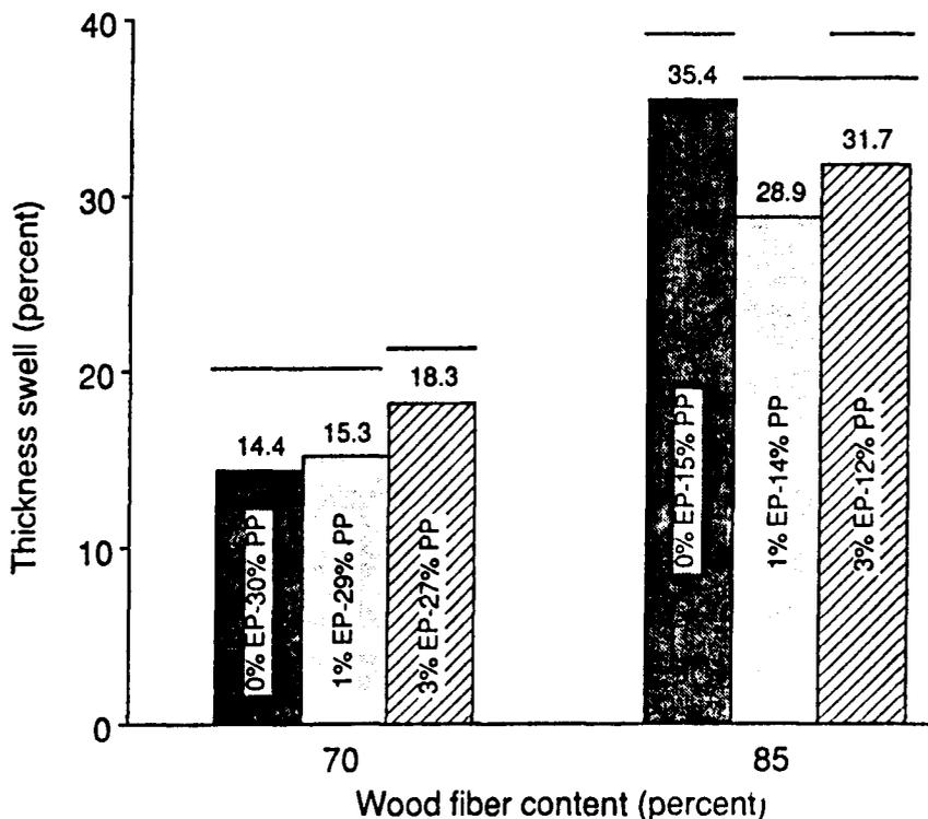
Figure 6. — 2-hour water-boil thickness swell of nonwoven web composite as a function of wood fiber content and MAPP-2 level. (EP is MAPP-2; PP is polypropylene; percentages are weight percent of total system. Bars connected by a solid line are not significantly different at the 95% confidence level.)
