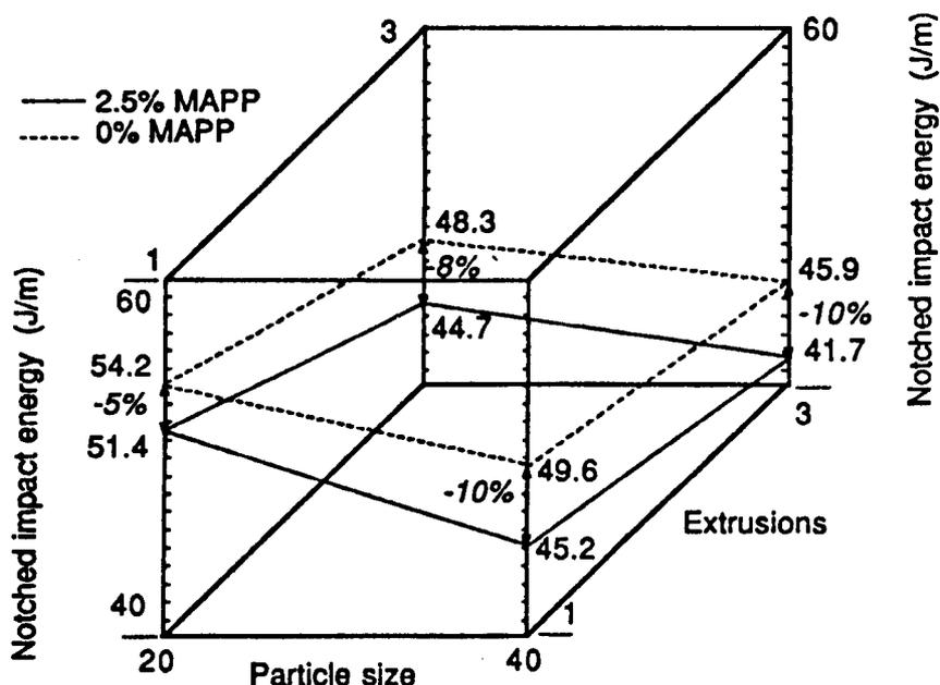
Figure 3. — Notched impact energy of extruded composite as a function of wood flour particle size, number of extrusions, and MAPP-1 level. (All data points are the average of results for one and three extrusions. MAPP levels are weight percentages of total system.)
