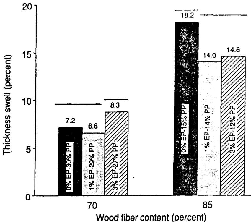
Figure 5. — 24-hour water-soak thickness swell of nonwoven web composite as a function of wood fiber content and MAPP-2 level. (EP is MAPP-2; PP is polypropylene; percentages are weight percent of total system. Bars connected by a solid line are not significantly different at the 95% confidence level.)
