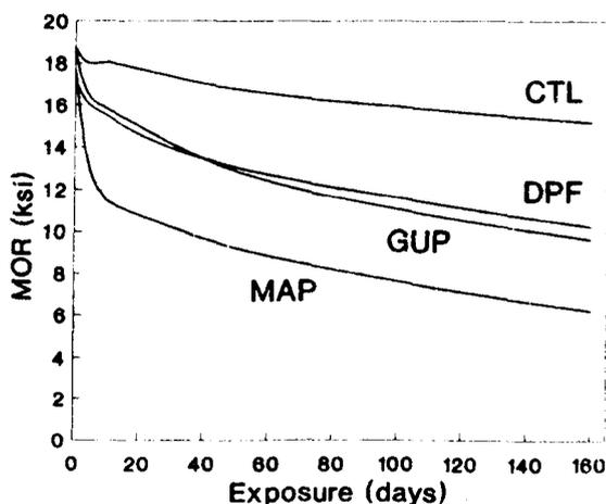
Figure 1. Effects of three fire retardants on bending strength of 0.625- x 1.375- x 12-in. clearwood specimens exposed to steady-state exposure at 180°F (82°C) and 50% RH (CTL = untreated control, MAP = monoammonium phosphate, GUP = guanidurea phosphate, and DPF = dicyandiamide phosphoric acid formaldehyde).
