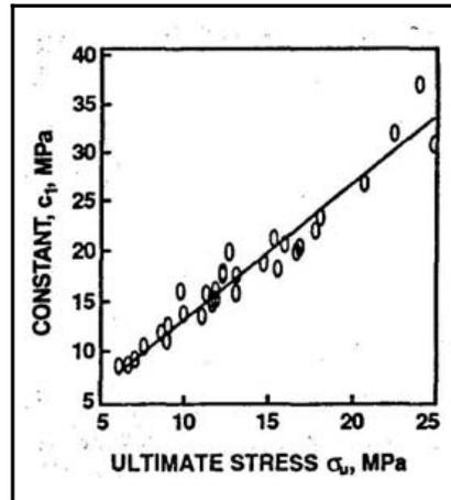
6. Comparison between the edgewise compressive strength of corrugated fiberboard predicted according to Eq. 18 and measured
