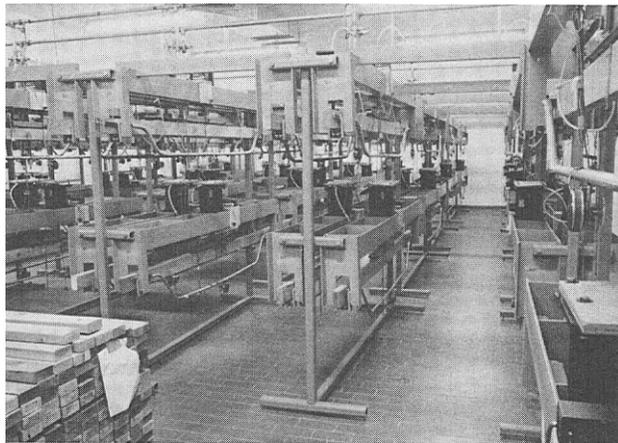
Figure 1. – Test frame setup for both static strength and constant load tests.
