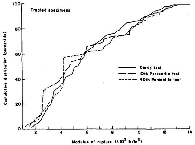
Figure 3. - Strength distributions for static strength test and constant load tests at the 10th and 40th percentiles of the static strength distribution for untreated and treated specimens.
