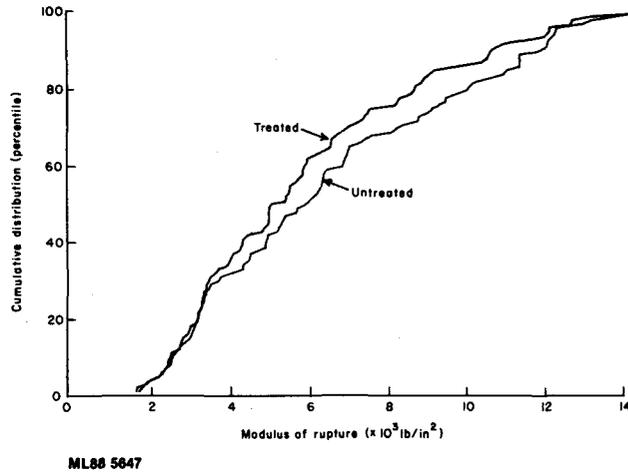
Figure 2. - Static strength distribution for treated and untreated control specimens.
