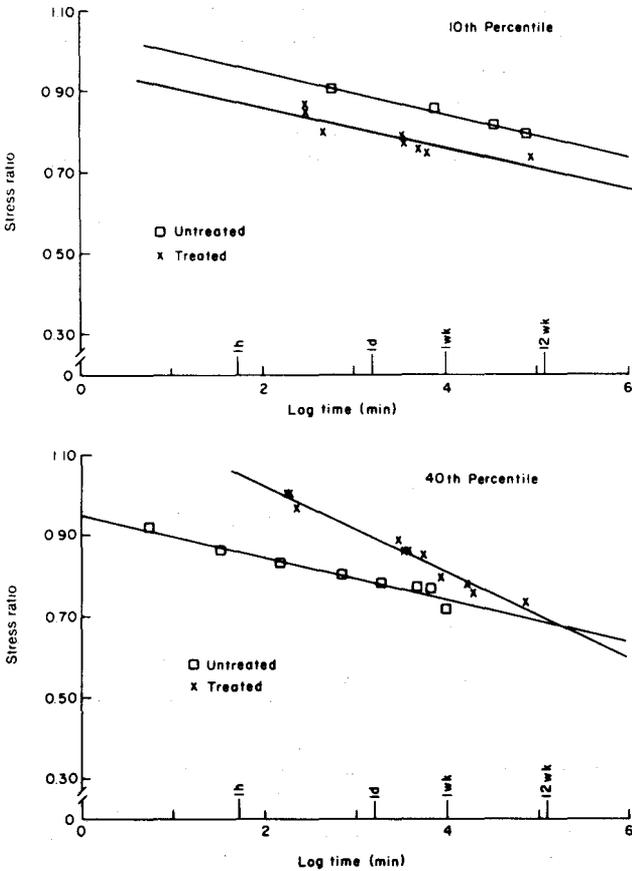
Figure 4. – Duration-of-load curves showing strength ratio on log time for constant loads at 10th and 40th percentiles of static strength.
