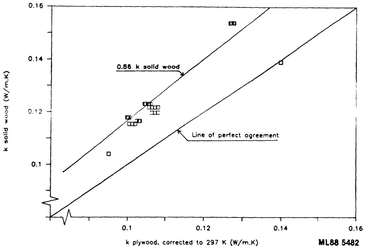
Fig. 8. Comparison of measured thermal conductivity of plywood with calculated values for solid wood (Eq. (7)) with the same density and MC. The data have been corrected for temperature.
