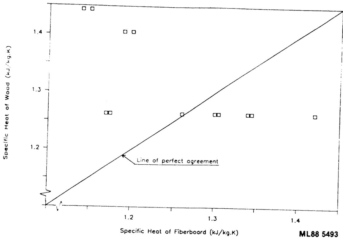
Fig. 14. Comparison of measured specific heat of fiberboard with calculated values for solid wood with the same density.
