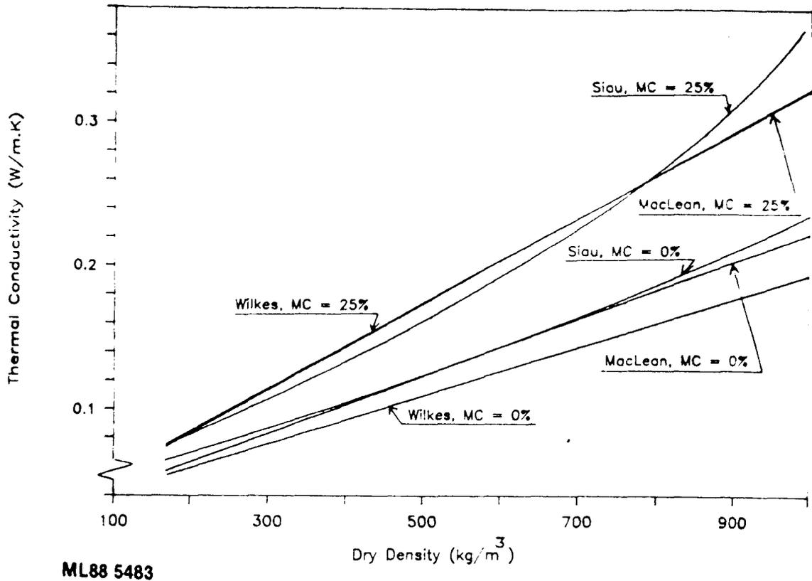
Fig. 4. Comparison of three alternative equations for conductivity of solid wood at 0 and 25 percent MC.
