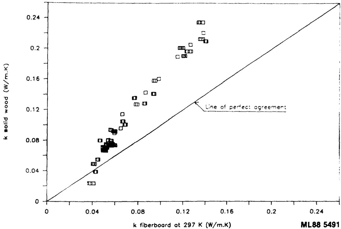
Fig. 12. Comparison of the measured thermal conductivity of fiberboard with calculated values for solid wood of the same density and MC.
