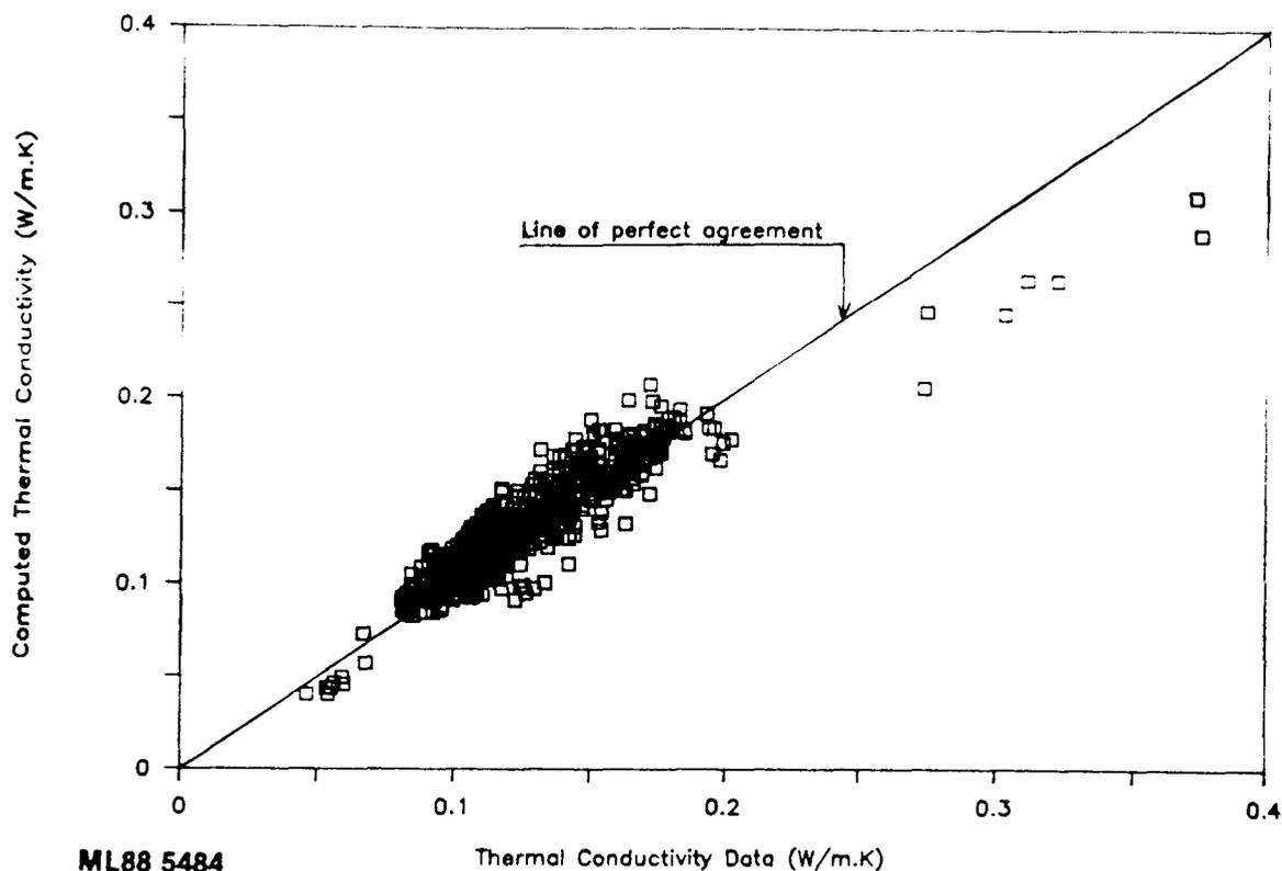
Fig. 5. Comparison of calculated conductivity of solid wood (Eq. (7a)) with conductivity data. All data on conductivity across the grain are included.
