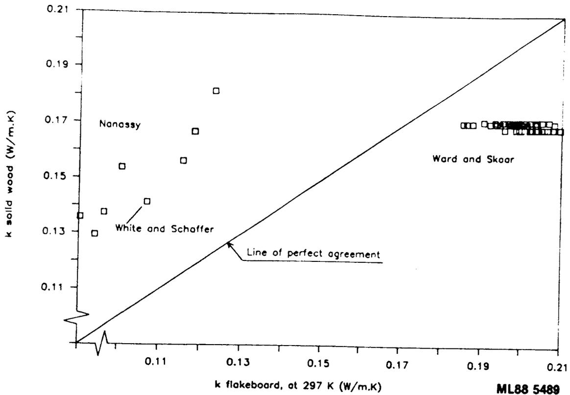
Fig; 10, Comparison of measured thermal conductivity of flakeboard with calculated values for solid wood with the same density and MC. The data has been corrected for temperature.
