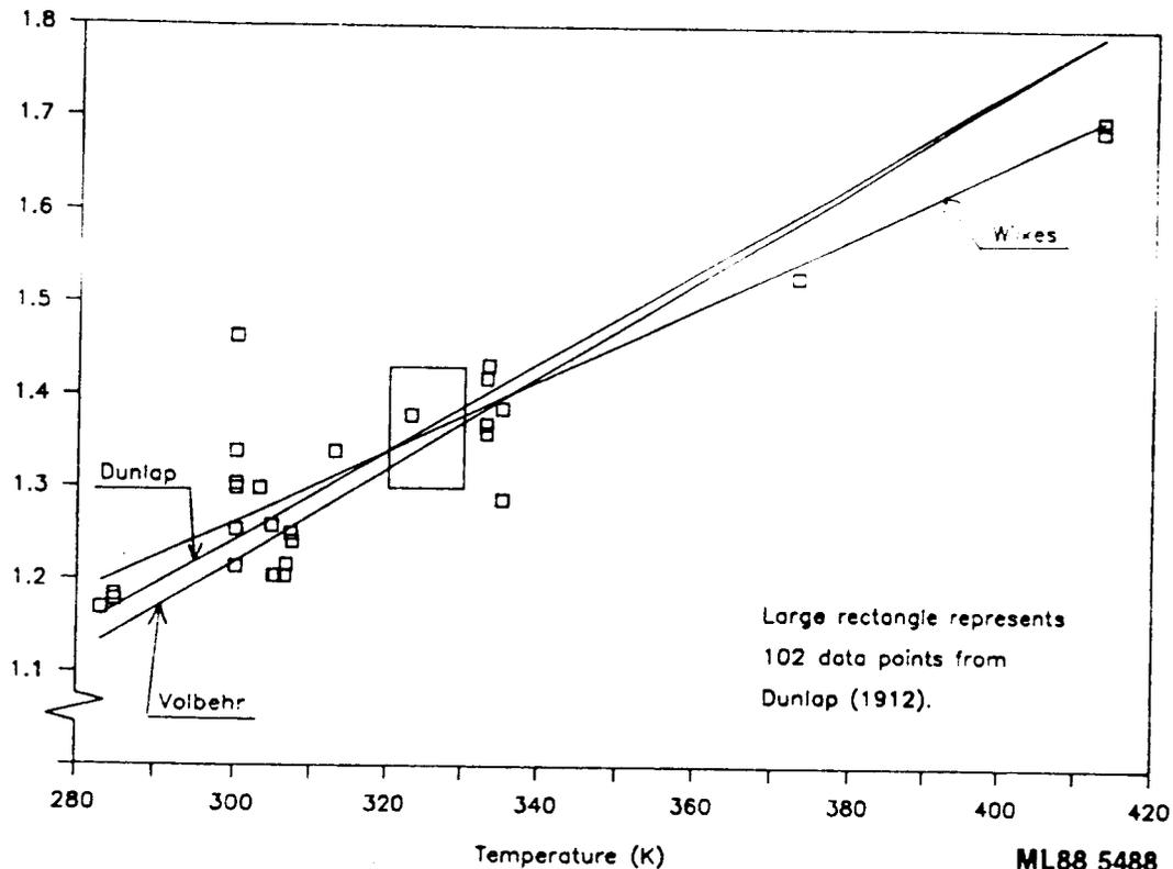
Fig. 7. Comparison of equations for specific heat of oven-dry solid wood at 0 MC.
