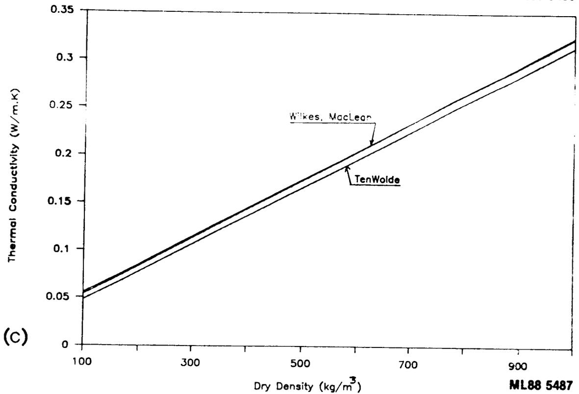
Fig. 6. Comparison of equations for conductivity of solid wood at (a) 0, (b) 12 percent, and (c) 25 percent MC.
