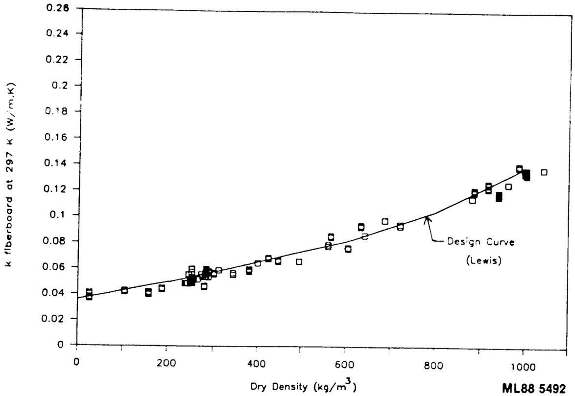
Fig. 13. Thermal conductivity of fiberboard as a function of dry density, compared with design values proposed by Lewis (1).
