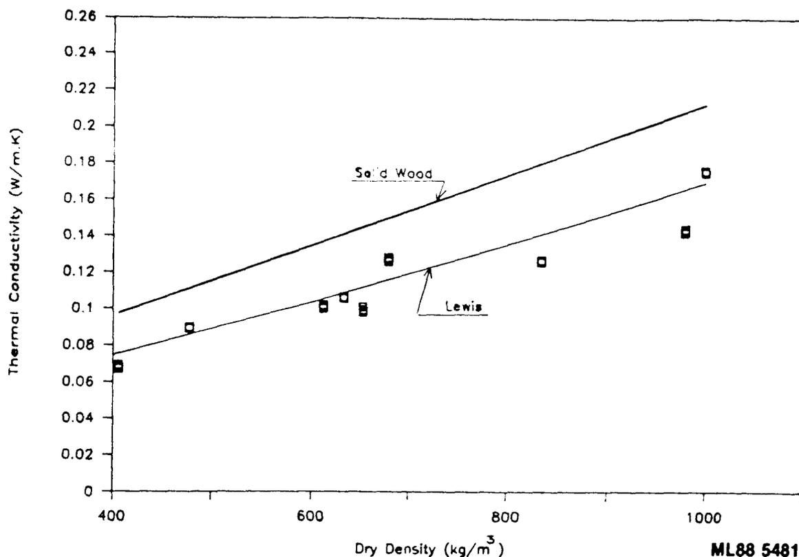
Fig. 9. Comparison of design values for thermal conductivity of dry particleboard proposed by Lewis (1) with measured values for dry particleboard and with calculated values for ovendry solid wood with the same density.
