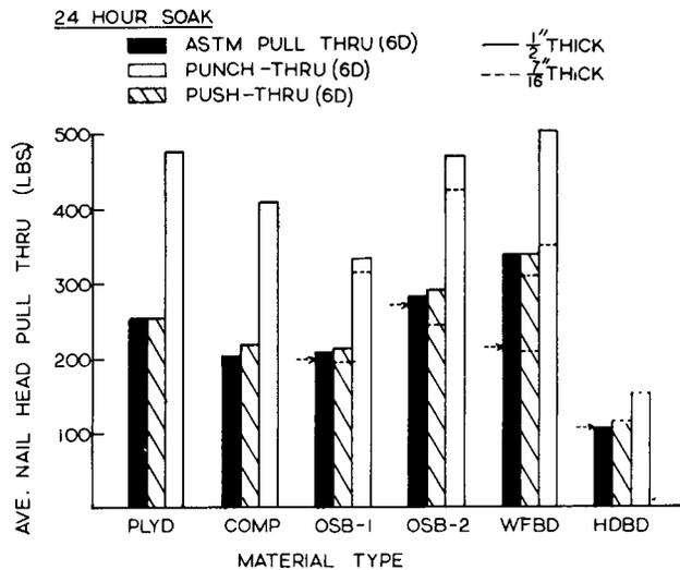
Figure 7. — The effects of three test methods on nailhead pull-through resistance of six wood-based materials with two thicknesses (24-hr. water-soaked condition).
