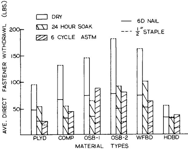
Figure 5. — The average direct 6-penny nail and 1/2-inch staple withdrawal resistance of six wood-based materials at three exposure conditions.
