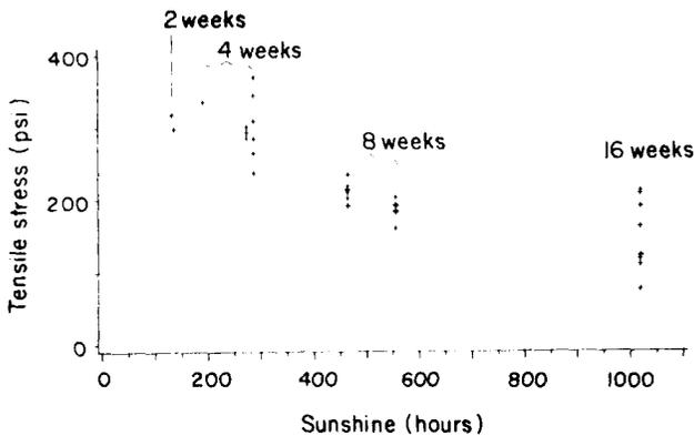
Figure 1. — Ultimate tensile stress (psi) versus wood weathering time (hr. of sunshine) of acrylic latex primer paint coated on western redcedar. Only primer/wood interface failures are shown.
