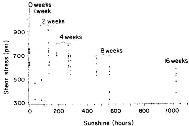
Figure 2. — Ultimate shear stress (psi) versus wood weathering time (hr. of sunshine) of alkyd oil primer paint on western redcedar. Only primer/wood interface failures are shown.
