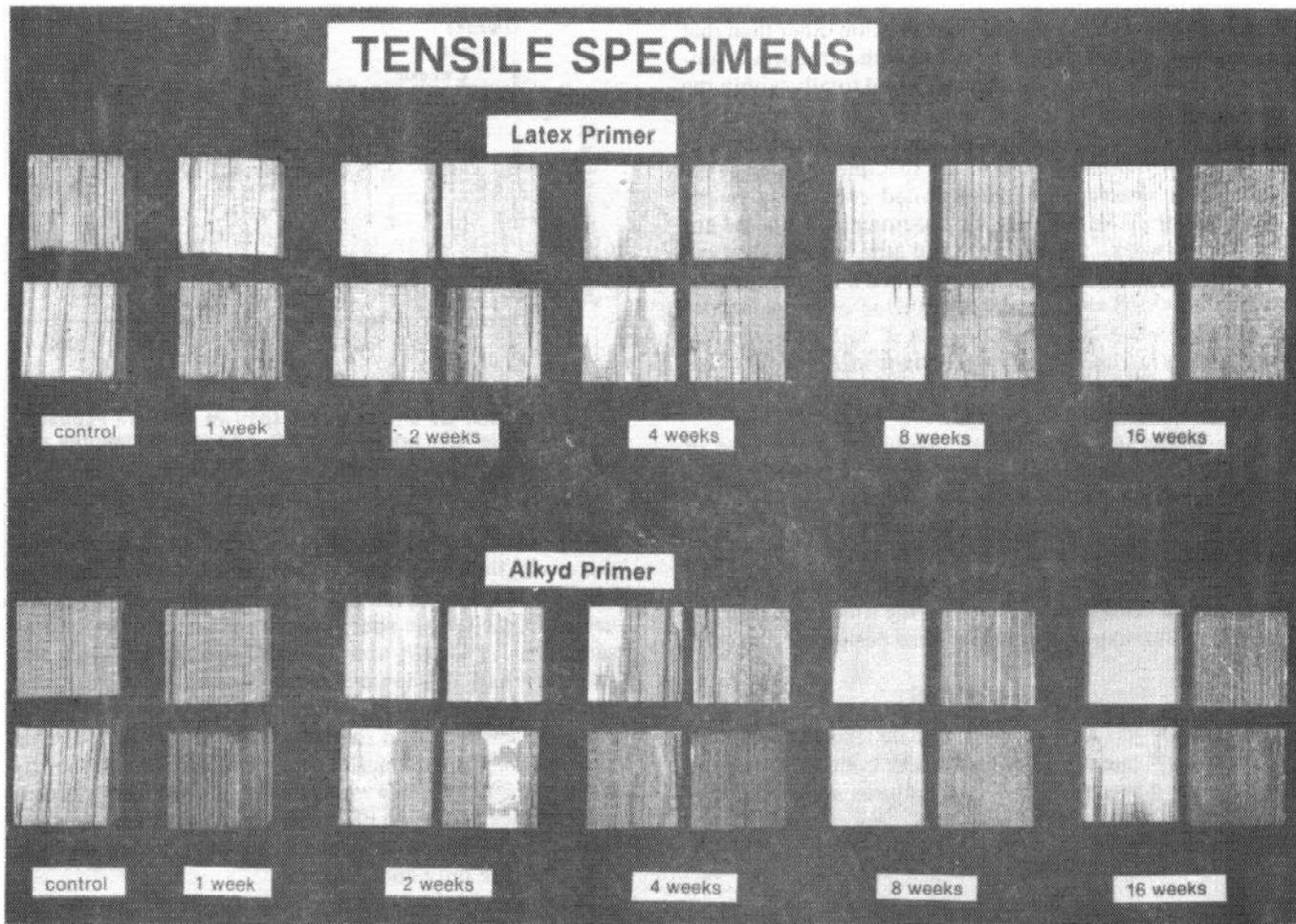
Figure 5—Failure surfaces of representative tensile specimens. (M86 0043)
