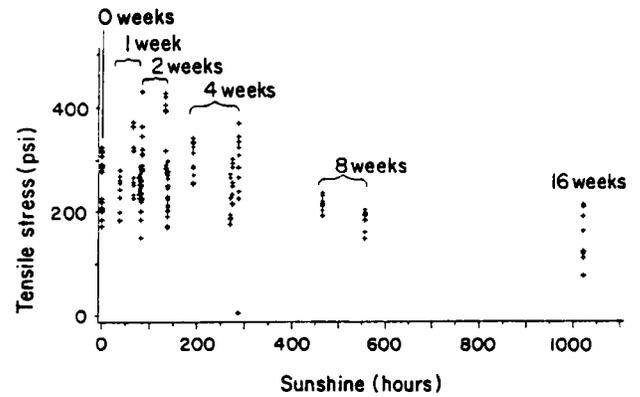
**Figure 4— Ultimate tensile stress (psi) vs sunlight exposure time of acrylic latex primer on WRC. All adhesive failures and cohesive wood failures are shown. (ML86 5259)**
