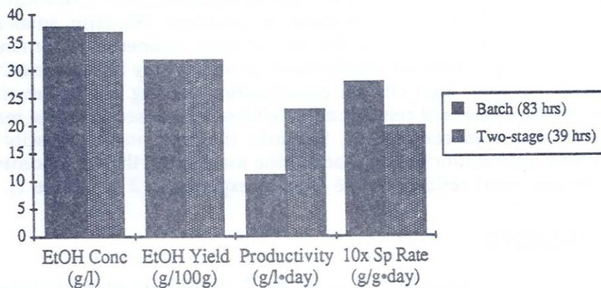
Fig. 3. Comparison of batch culture with the two-stage process. Batch culture is compared with the two-stage process. The batch example represented the maximum ethanol obtained from 12% xylose at 25°C. The fermentation time for the two stage reactor was the sum of the residence times of both reactors. The yield and productivity entries for the two stage reactor are overall values for both reactors combined.
