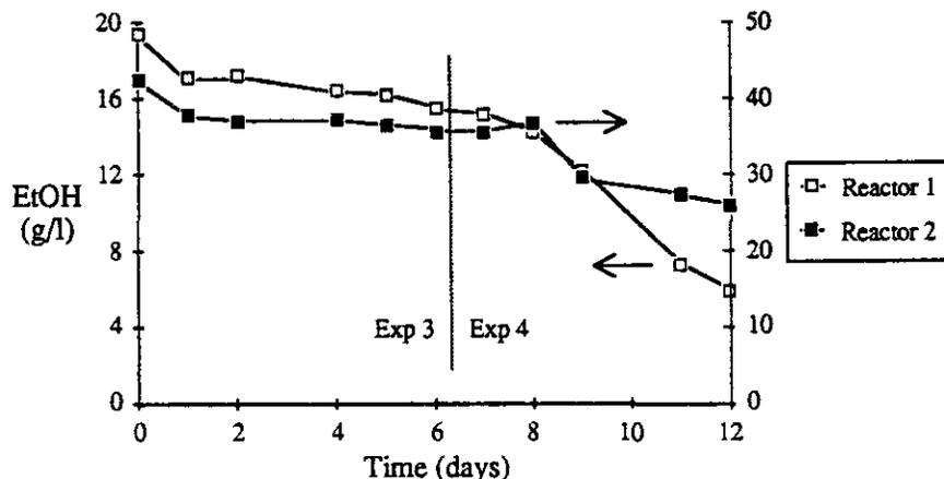
Fig. 2. Comparison of reactor stability of both reactors. Time profiles of ethanol concentration in both reactors are shown for experiments 3 and 4. The dilution rate of reactor 2 was changed from 0.035 h<sup>-1</sup> to 0.025 h<sup>-1</sup> between experiment 3 and 4. No change was made in operating conditions for reactor one; the dilution rate remained constant at 0.096 h<sup>-1</sup>.
