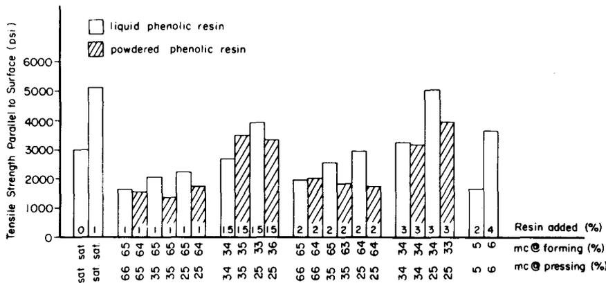
Figure 4. — Tensile strength parallel to surface.
