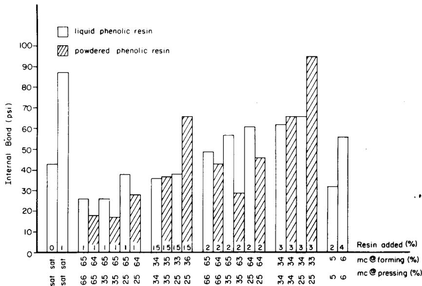
Figure 5. — Tensile strength perpendicular to surface (internal bond).
