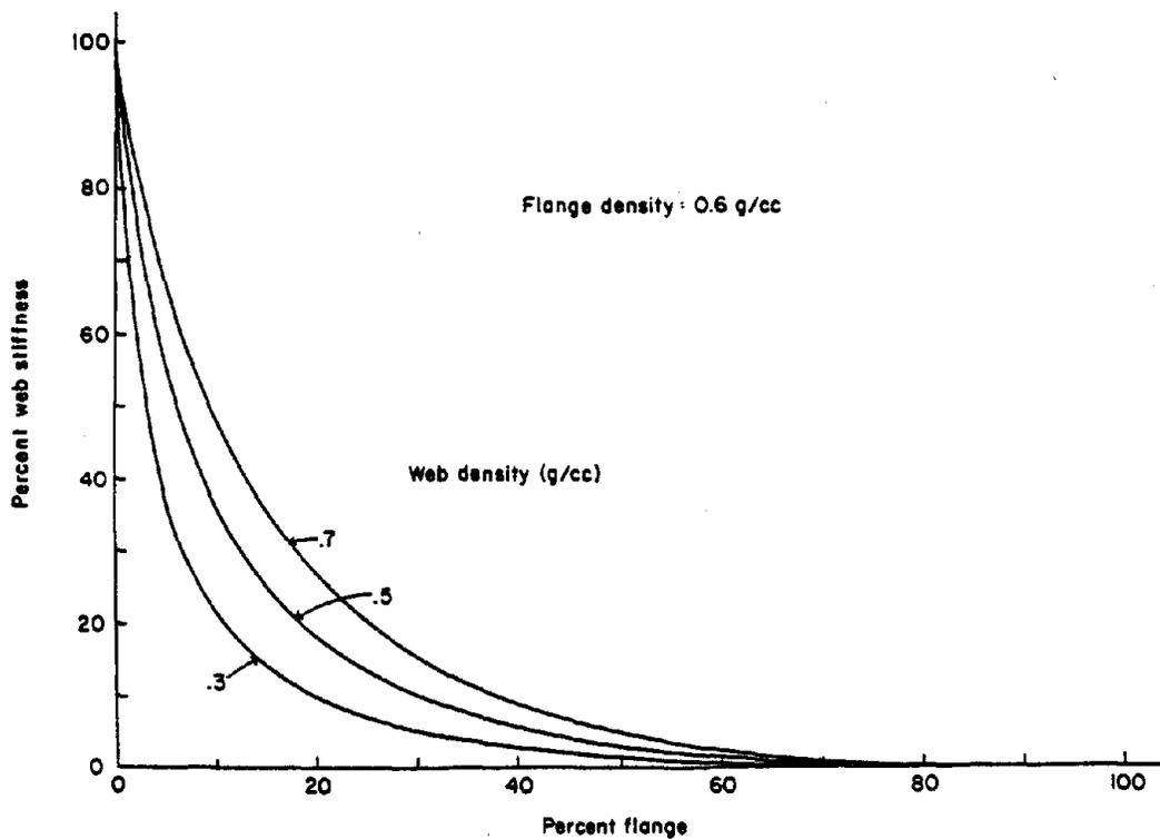
Figure 2.--Contribution of the web-to-beam stiffness with alignment and flake-type uniform throughout beam
