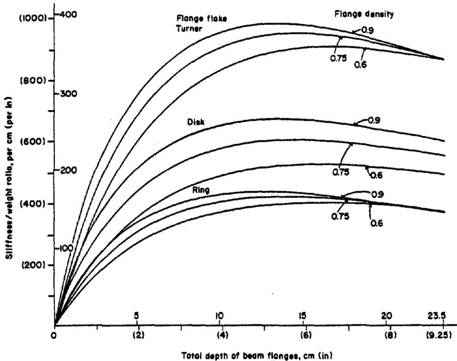
Figure 3.—Results of optimization for 6 m (20 ft) span, uniformly loa loaded, 3.8 by 23.5 cm (1.5 by 9.25 in.) composite beam
