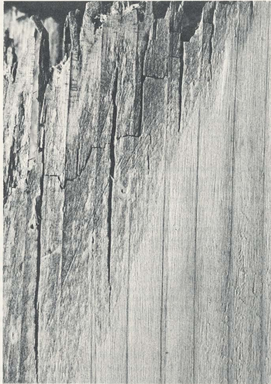
FIG. 1. Brown rot by an unidentified fungus in heartwood of a WRC pole. Note typical checking across the grain and narrow zone of transition between decay and sound wood.
