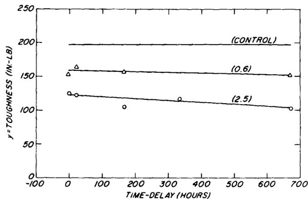
Figure 3. — Effects of time-delay (hours) on the toughness of small clear specimens of southern pine. Estimated regression equation for CCA-treated southern pine at 0.6 pcf is  $y = 158.152 - 0.0105(x)$  ( $R^2=0.005$ ) and for 2.5 pcf is  $y=122.389 - 0.0273(x)$  ( $R^2 = 0.049$ ) where  $y$  = toughness (in.-lb.) and  $x$  = time-delay (hr.).
