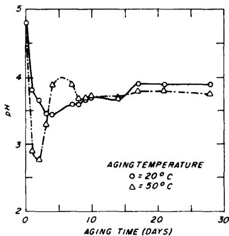
Figure 1. — The pH curve during aging of precipitate from Boliden  $K_{33}$  (CCA type B). (All measurements carried out at 20°C.) From (8).
