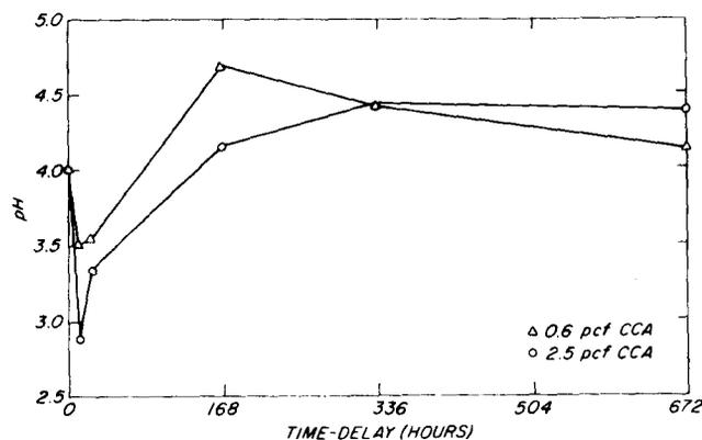
Figure 2. - Variation of wood pH due to increasing periods of time delay for small clear specimens of southern pine treated to two CCA retention levels.
