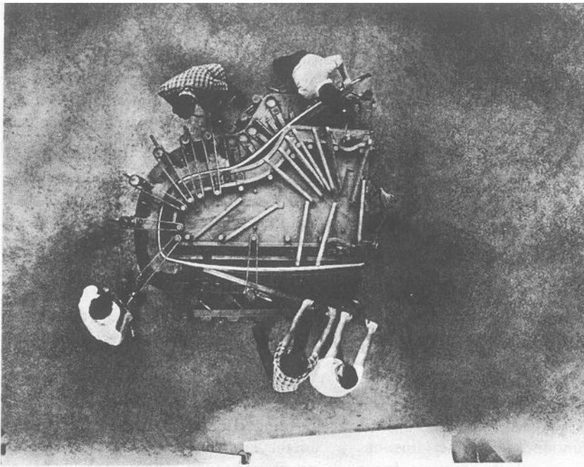
**Figure 7.** Bending the rim of a grand piano, using as many as 22 continuous layers of selected eastern rock maple wood, is the method used over the last hundred years by a famous firm of piano makers. (Courtesy Steinway and Sons, New York.)
