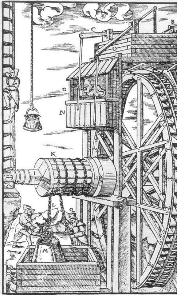
**Figure 3.** Wooden macro-engineering in the 16th century. Agricola in his *De re metallica*, Basle (1556), produced the first mining technology work and here illustrated is a reversible hoist for raising ore from a shaft. The operator, O, in his hut, N, through levers C and D can regulate the water flow, B, to fall on wheel E or F, thus rotating it in either direction. The leather bucket M can thus be raised or lowered. (Ann Ronan Picture Library.)
