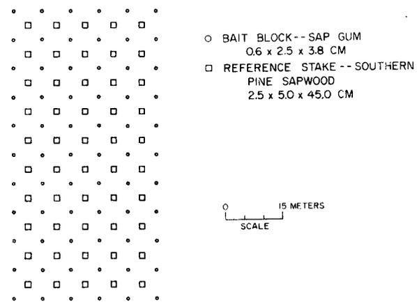
FIG. 2. — Placement of 66 bait blocks (o) and 50 southern pine stakes (□)/plot.
