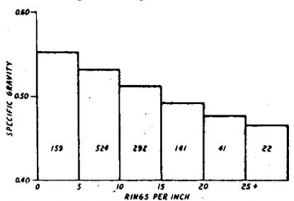
Figure 3.--Relationship of specific gravity to rate of growth (rings per inch) of all black walnut specimens by growth rate classes. The height of each bar represents the average specific gravity found from tests on the number of specimens indicated in each bar having a ring count falling in the class interval shown at the bottom of each bar. Specific gravity values in this figure are based upon the weight of the specimens when oven dry and their volume when green.
