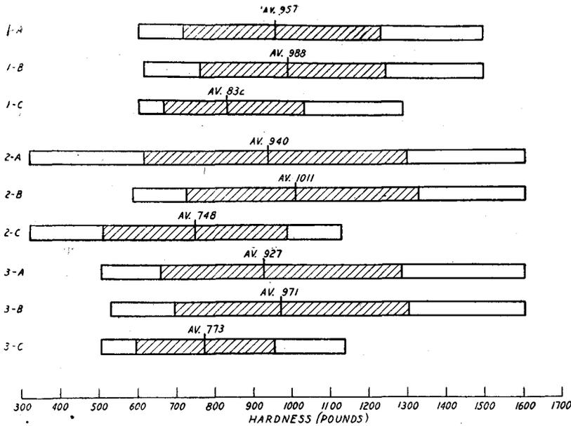
Figure 5—Variation in hardness, for end, tangential, and radial surfaces and separately for sapwood and heartwood of each surface at all heights in open-grown and forest-grown black walnut trees tested in a green condition
