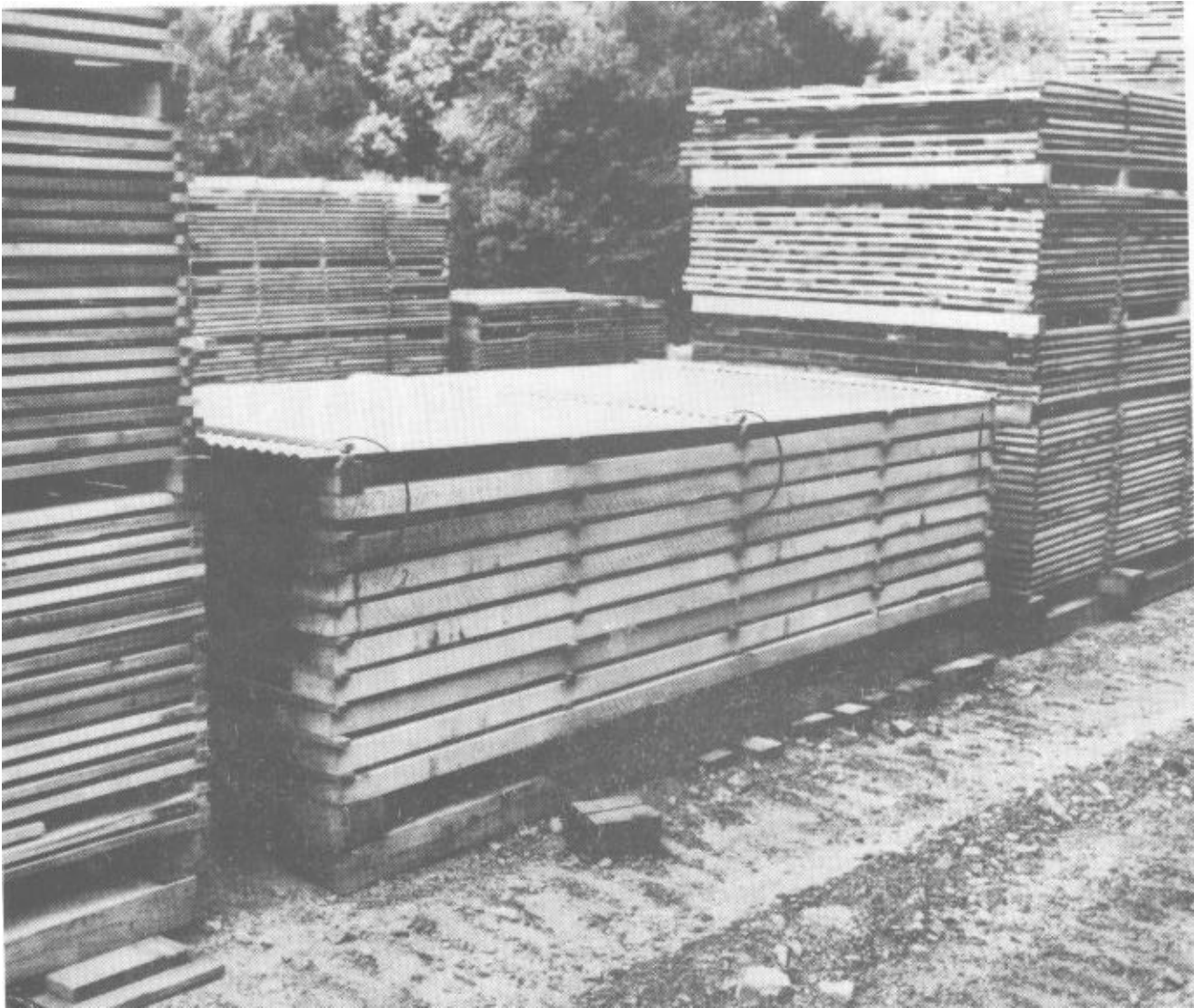
Figure 1.-- This illustrates correct stacking. Note that the bottom layer is well above the ground, stickers are directly above one another, ends of the boards are in contact with a sticker, and a pile cover is in use and tied down.
