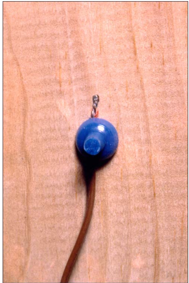
Figure 4—Surface thermocouple held in place by push pin.
