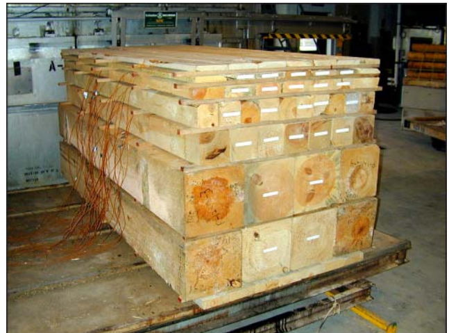
Figure 5—Stack of boards and timbers ready to be pushed into the kiln for heating. Pieces with white tags have thermocouples.
