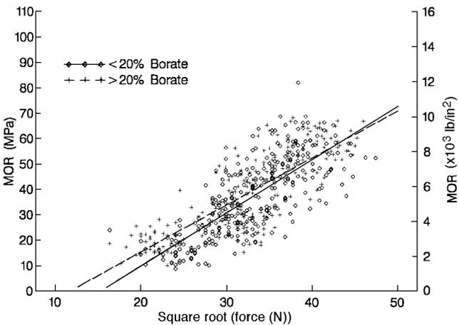
**Figure 10—Example of how combined groups could have significantly different regressions but support the same general effect on bending strength of 16-mm- (5/8-in.-) thick plywood (Winandy, in progress; 1997).**
