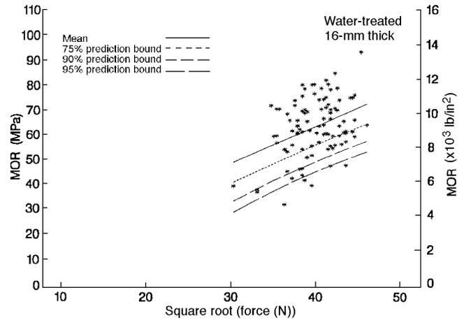
**Figure 17—Mean trends and lower prediction bounds for relationship of screw-withdrawal force to bending strength for water-treated 16-mm- (5/8-in.-) thick plywood in both Lab-Field and Factors studies (Winandy, in progress; Winandy 1997).**
