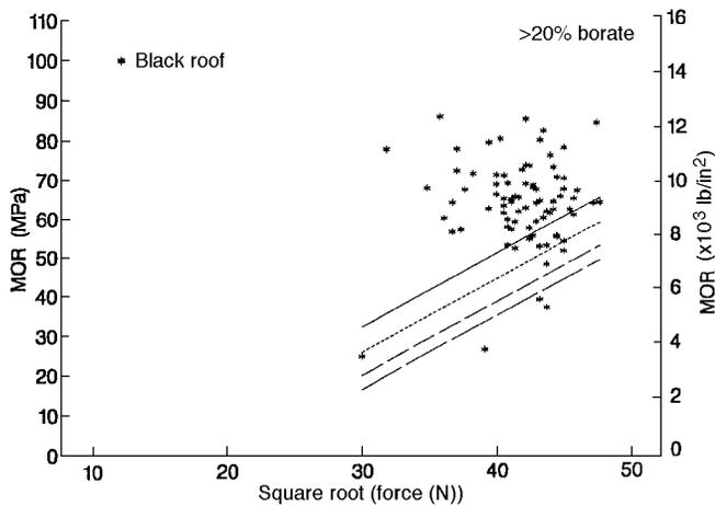
**Figure 20—Example of applicability of models as shown by predicted mean trends and lower prediction bounds compared to real data from material treated with MAP and >20% borate. Real data were obtained from treated 16-mm- (5/8-in.-) thick material exposed in the field for 1 year; these data were not used to develop the model parameters (Winandy, in progress).**
