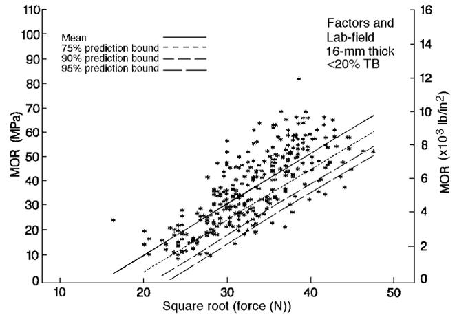
**Figure 13—Mean trends and lower prediction bounds for relationship of screw-withdrawal force to bending strength for 16-mm- (5/8-in.-) thick plywood treated with MAP/<20% borate (Winandy, in progress; Winandy 1997).**
