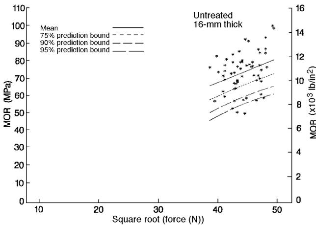
**Figure 16—Mean trends and lower prediction bounds for relationship of screw-withdrawal force to bending strength for untreated 16-mm- (5/8-in.-) thick plywood in both Lab-Field and Factors studies (Winandy, in progress; Winandy 1997).**
