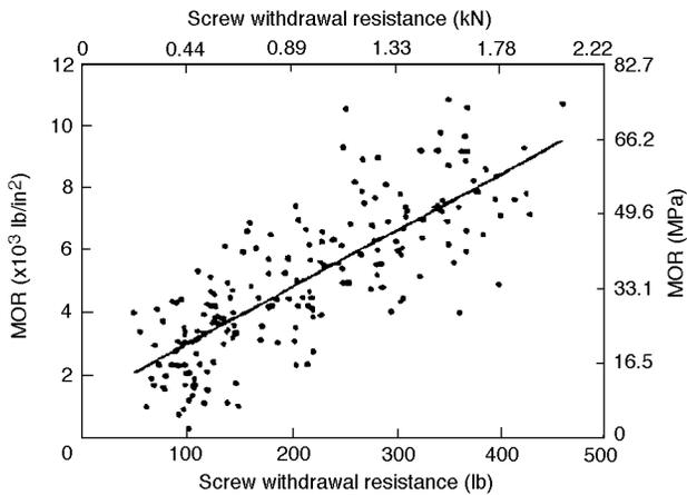
**Figure 2—Relationship of bending strength (modulus of rupture) to screw withdrawal resistance—Ross and others 1992.**
