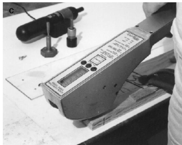
**Figure 4—Screw-withdrawal test. Battery-powered screwdriver and jig are used to drill pilot hole (A) and insert screw (B); screw-extraction-force tool is used to withdraw screw while peak withdrawal force is monitored (C).**
