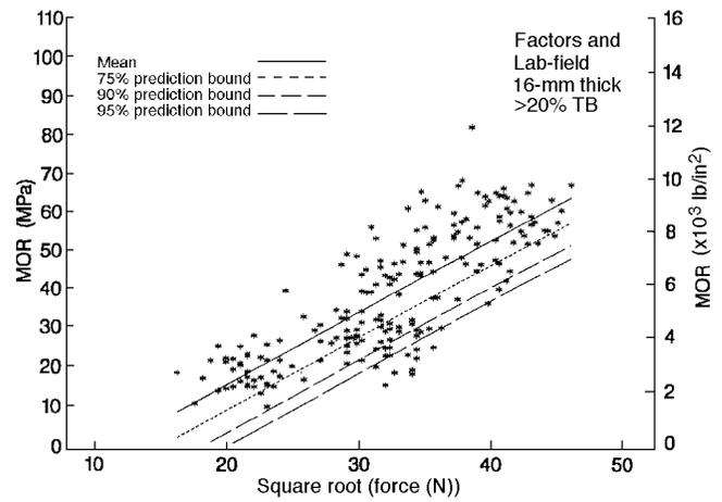
**Figure 14—Mean trends and lower prediction bounds for relationship of screw-withdrawal force to bending strength for 16-mm- (5/8-in.-) thick plywood treated with MAP/>20% borate (Lab-Field Study) and 80/10/10 and 80/0/20 groups of Factors Study (Winandy, in progress; Winandy 1997).**
