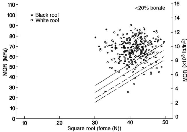
**Figure 19—Example of applicability of models as shown by predicted mean trends and lower prediction bounds compared to real data from material treated with MAP and <20% borate. Real data was obtained from treated 16-mm- (5/8-in.-) thick material exposed in the field for 1 year; these data were not used to develop the model parameters (Winandy in progress).**
