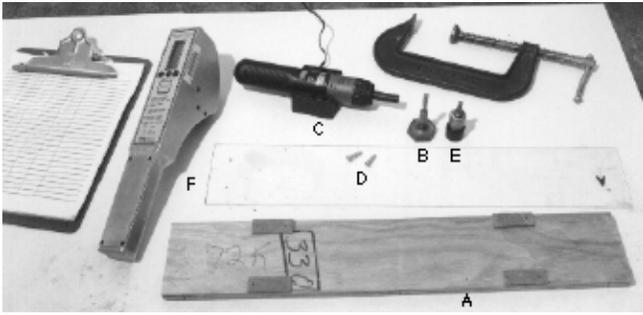
**Figure 3—Specimen and equipment for screw-withdrawal test: (A) plywood specimen, (B) 3.1-mm- (1/8-in.-) diameter drill bit, (C) battery-powered screwdriver, (D) 22-mm- (7/8-in.-) long No. 10 wood screws, (E) jig, and (F) screw-extraction-force tool.**
