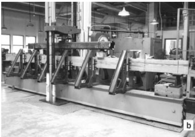
Figure 5—Configuration of test equipment showing (a) location and load points, support reactions, and lateral supports. Actual single-ply (b) and four-layer (c) specimens are shown prior to tests. (M92 0030–12, 0016–4)
