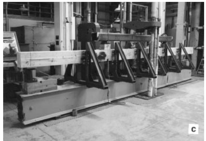
Figure 5—Configuration of test equipment showing (a) location and load points, support reactions, and lateral supports. Actual single-ply (b) and four-layer (c) specimens are shown prior to tests. (M92 0030–12, 0016–4)
