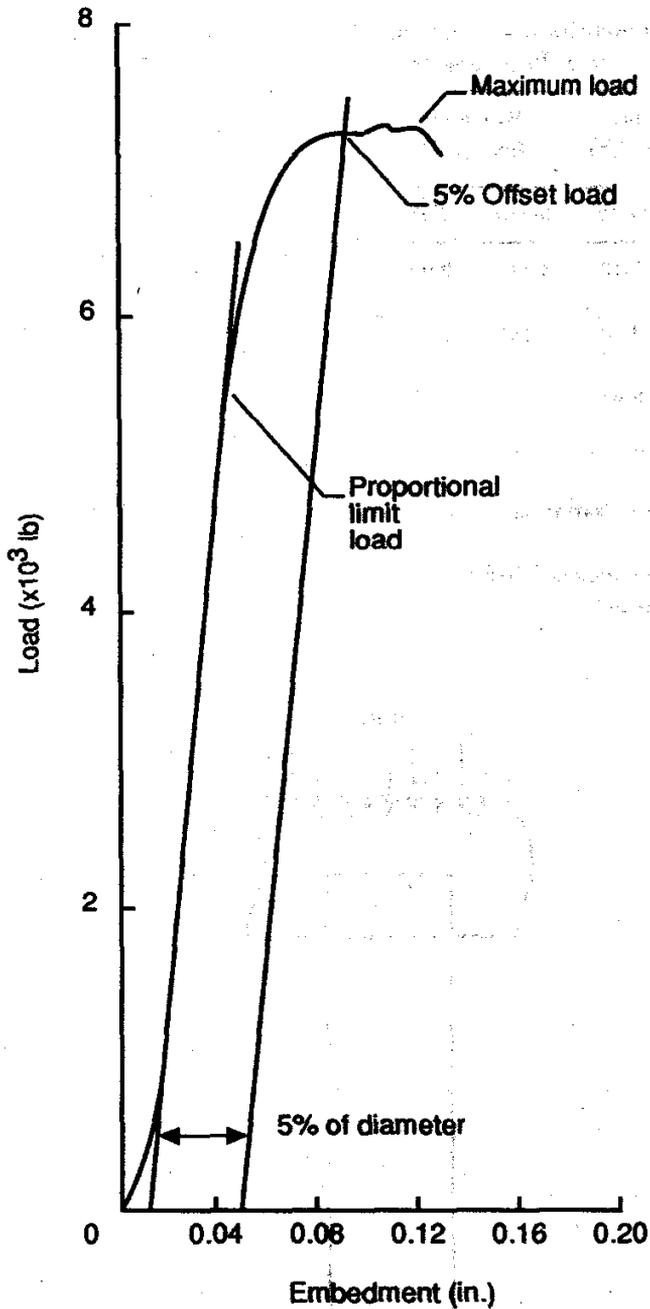
Figure 2—Typical load-embedment curve for a 3/4-in. (19-mm) bolt loaded parallel to grain in Southern Pine (1 in. = 25.4 mm; 1 lb = 4.45 N). Tabulated loads are indicated on the curve.
