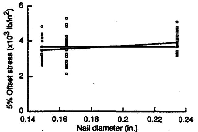
Figure 10—Relation between dowel bearing strength and nail diameter for Douglas Fir for both loading directions (1 in. = 25.4 mm; 1 lb/in<sup>2</sup> = 6.89 kPa). Nail bearing strength multiplied by 0.38  $G_1^{1.84}$ .
