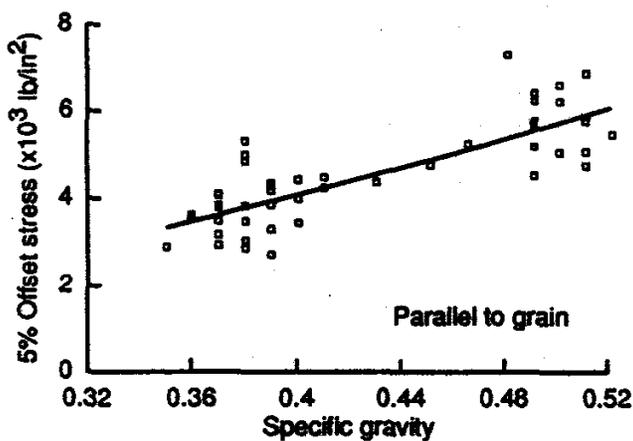
Figure 7—Relation between dowel bearing strength and specific gravity  $G_{12}$  for 0.162-in. (4.1-mm) nails loaded parallel to grain (1 lb/in<sup>2</sup> = 6.89 kPa).
