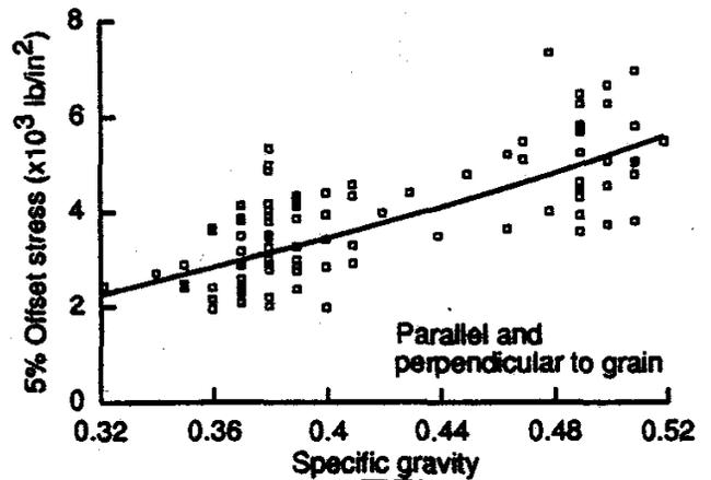
Figure 9—Relation between dowel bearing strength and specific gravity  $G_{12}$  for 0.162-in. (4.1-mm) nails, combining both loading directions (1 lb/in<sup>2</sup> = 6.89 kPa).
