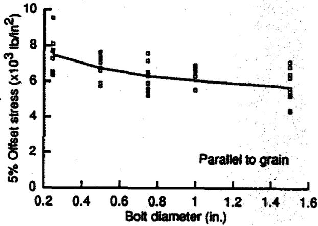
Figure 5—Relation between dowel bearing strength and bolt diameter for Southern Pine loaded parallel to grain (1 in. = 25.4 mm; 1 lb/in<sup>2</sup> = 6.89 kPa). Bolt bearing strength multiplied by a factor of 0.56/G<sub>12</sub>.
