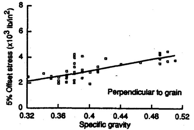
Figure 8—Relation between dowel bearing strength and specific gravity  $G_{12}$  for 0.162-in. (4.1-mm) nails loaded perpendicular to grain (1 lb/in<sup>2</sup> = 6.89 kPa).
