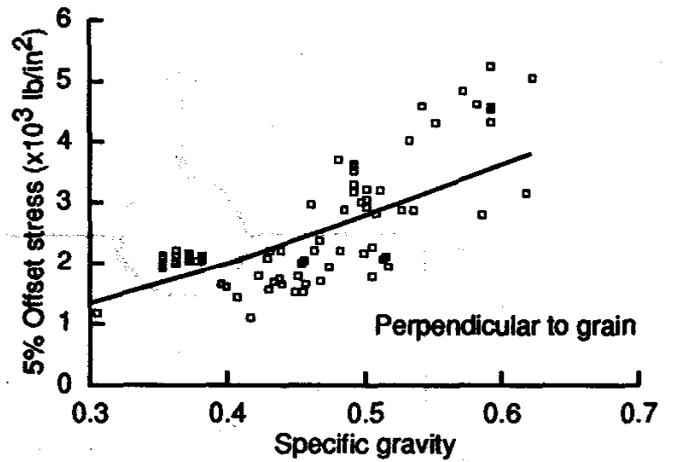
Figure 4—Relation between dowel bearing strength and specific gravity  $G_{12}$  for 3/4-in. (19-mm) bolts loaded perpendicular to grain (1 lb/in<sup>2</sup> = 6.89 kPa). The low values are from specimens from one board.
