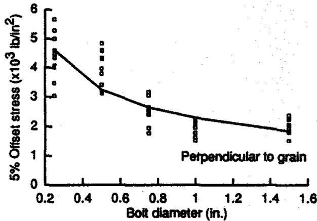
Figure 6—Relation between dowel bearing strength and bolt diameter for Southern Pine loaded perpendicular to grain (1 in. = 25.4 mm; 1 lb/in<sup>2</sup> = 6.89 kPa). Bolt bearing strength multiplied by a factor of 0.56/G<sub>12</sub>.
