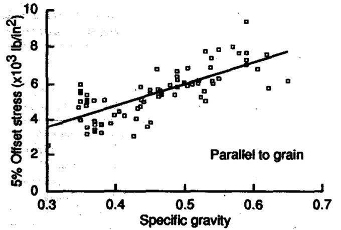
Figure 3—Relation between dowel bearing strength and specific gravity  $G_{12}$  for 3/4-in. (19-mm) bolts loaded parallel to grain (1 lb/in<sup>2</sup> = 6.89 kPa).
