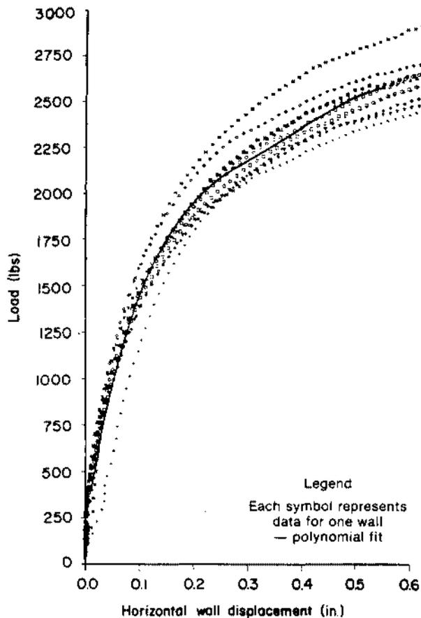
**Figure 5.--Load versus horizontal wall displacement for 10 plywood one-sided walls 4 feet in length with polynomial fit. Points from polynomials are used to compare wall types and lengths. (ML84 5248)**
