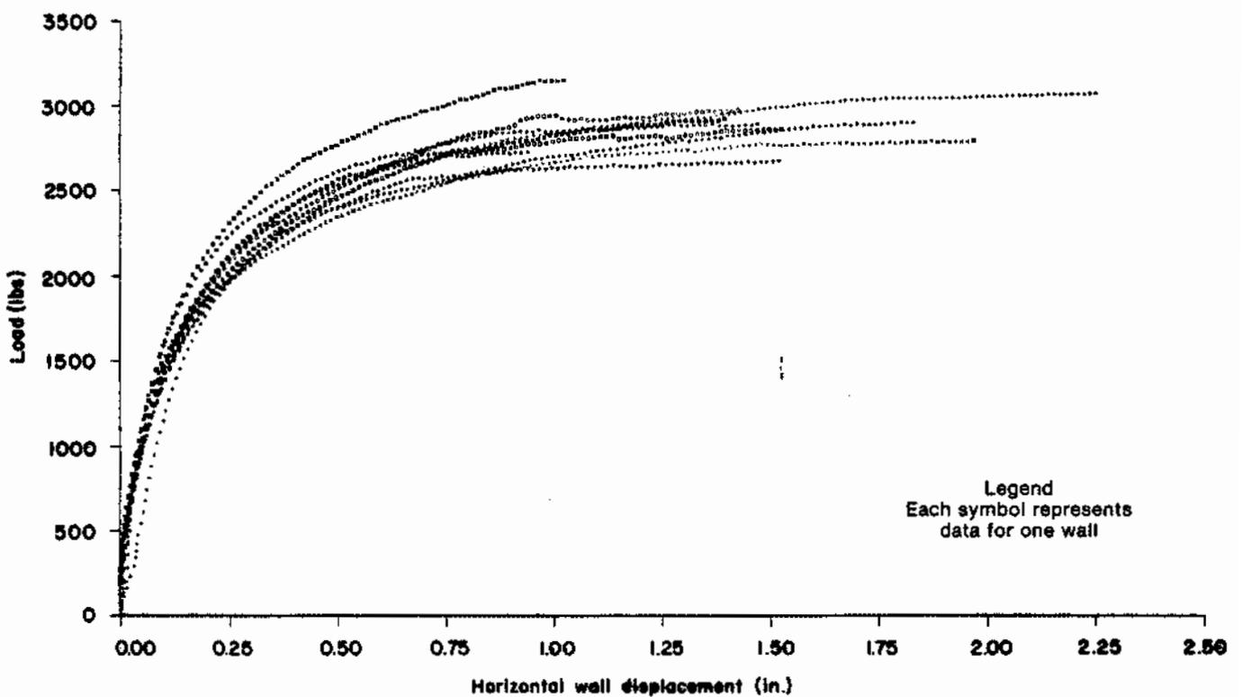
Figure 4.--Load versus horizontal wall displacement for 10 plywood one-sided walls 4 feet in length. (ML84 5247)
