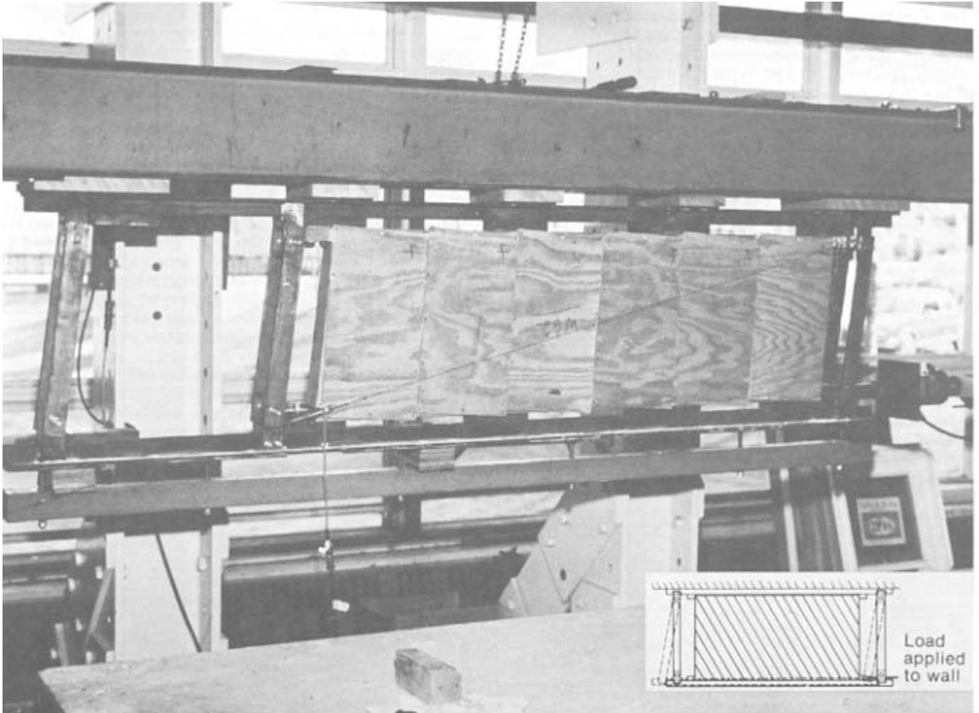
**Figure 3.--Test apparatus for wall racking tests. Test panel is 2 feet high by 6 feet long. Racking load is applied at lower right corner of frame. (M153003-11)**
