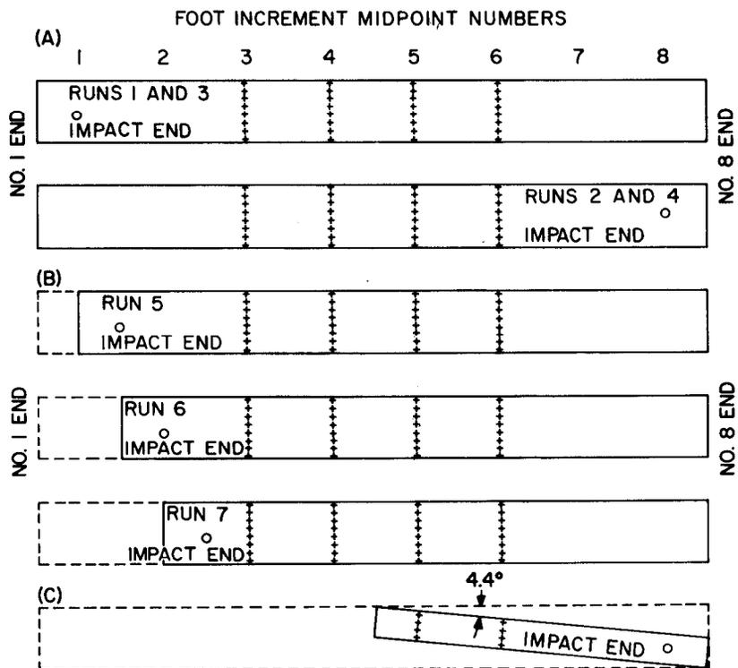
Figure 4.—Diagram showing impact end for runs and the grid points (+) to which transit times were measured. Circled dot indicates 8-inch position of first accelerometer from impact end. (A) 2 x 8's 8-foot length, 32 grid points; (B) 2 x 8's, consecutive 6-inch lengths removed, 32 grid points; (C) 2 x 4 cut from 2 x 8 with a 4.4° bias, 8 grid points. M 148 207
