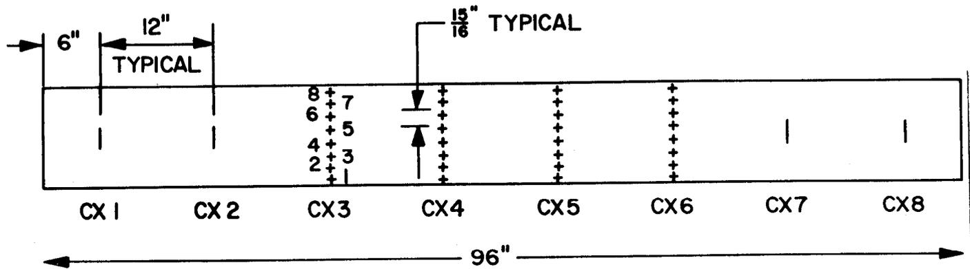
Figure 1.—Markings on the bark side of each specimen—The numbers 1 through 8 identify the midpoints of the 1-foot increments, which also mark the location of cross sections. Another set of numbers 1 through 8 identifies the locations of grid points set 15/16 inch apart on the cross sections. M 148 391
