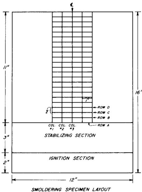
Figure 1.—Specimen with scribed grid for smoldering test.
