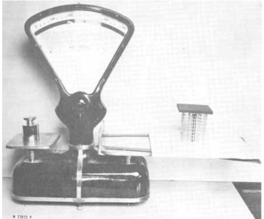
Figure B-2.—Apparatus for testing glow performance of insulation boards, showing test specimen in position.
