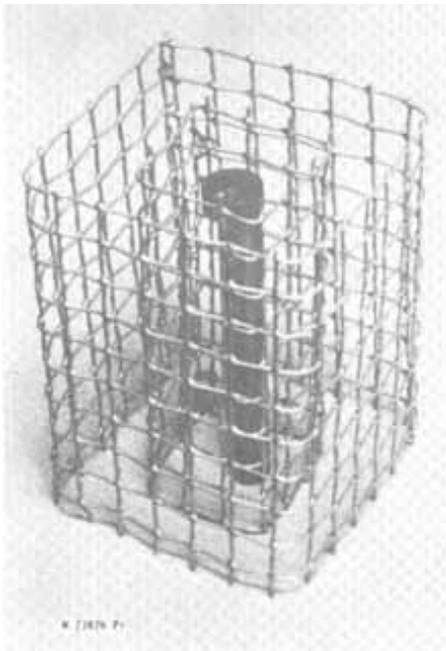
Figure B-1.—Apparatus for supporting test specimen and alcohol cup. Specimen to be supported on top wire strand.
