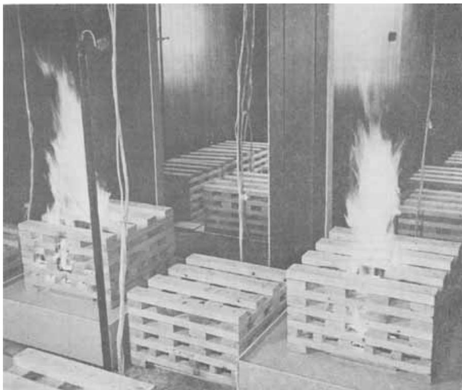
Figure 3.—Ignition cribs shortly after the start of the test—Structure 7. White, beaded wires are thermocouple "frees." Pipes at center of rear room and at the far left are for gas sampling.
