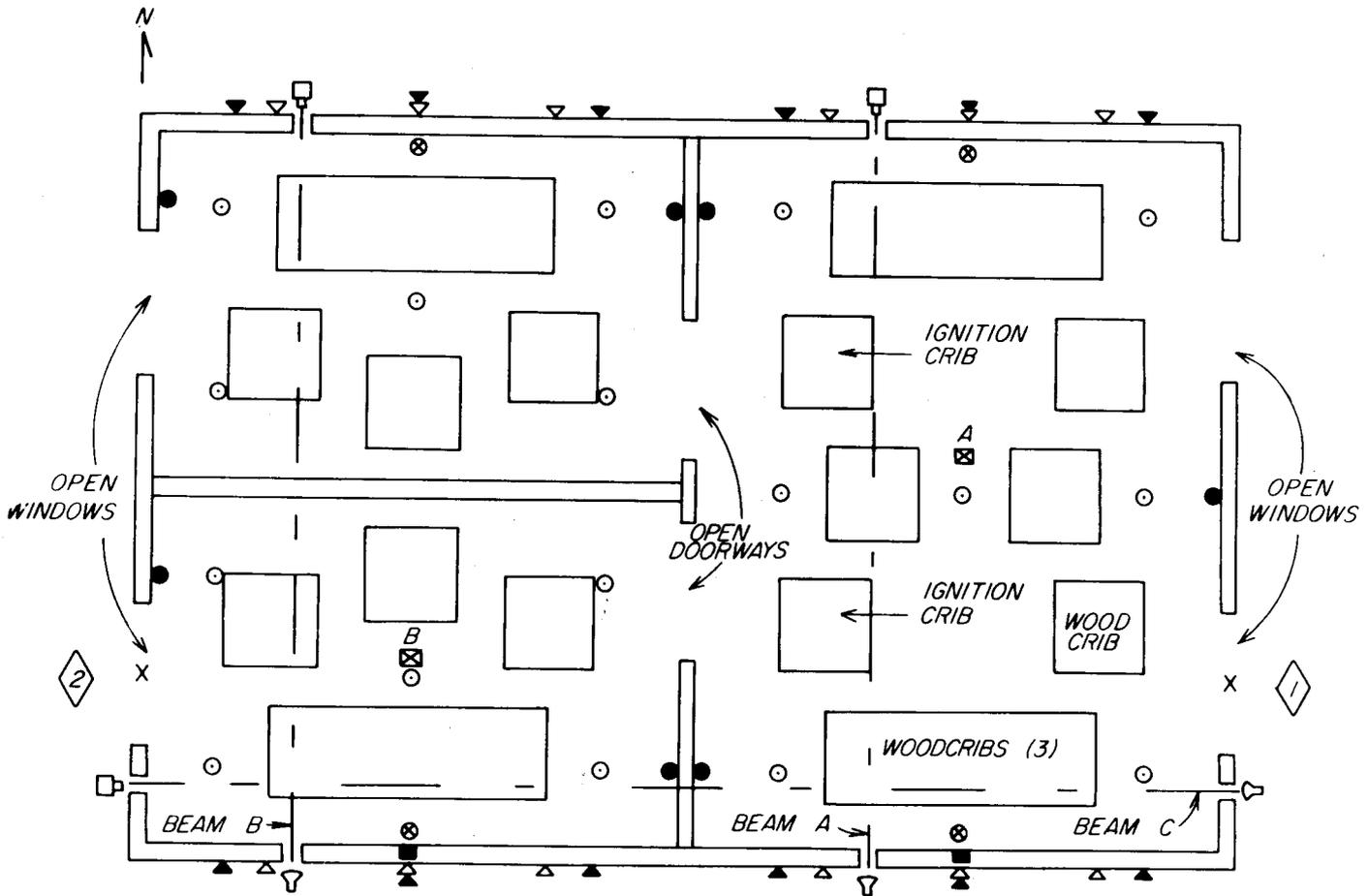
Figure 2.—Plan view of sandwich and wood-frame test structures showing locations of wood cribs, thermocouples, gas sampling points, and smoke-measuring apparatus.
