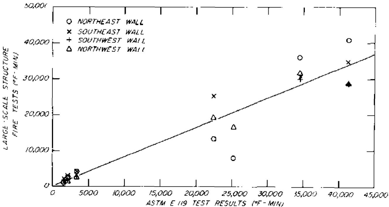
Figure 20.—Areas under the time-temperature curves (average of three protected thermocouples) from ignition to wall failure (see table 11). The two points with ASTM E 119 areas of 25,218° F·minutes are for Structure 2. Because of instrumentation difficulties, temperature data for Structure 2 are limited and erratic, and the accuracy of the areas is not known.
