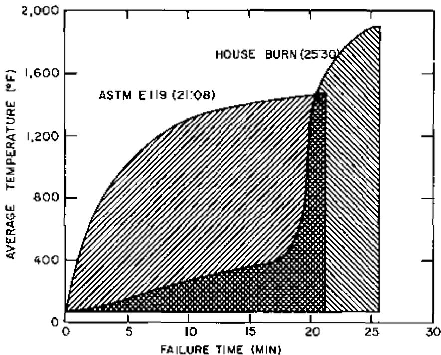
Figure 19.—Time-temperature relationship to time of structural failure for wall construction in ASTM E 119 laboratory test compared to first wall failure (northeast) in full-scale test of Structure 7.
