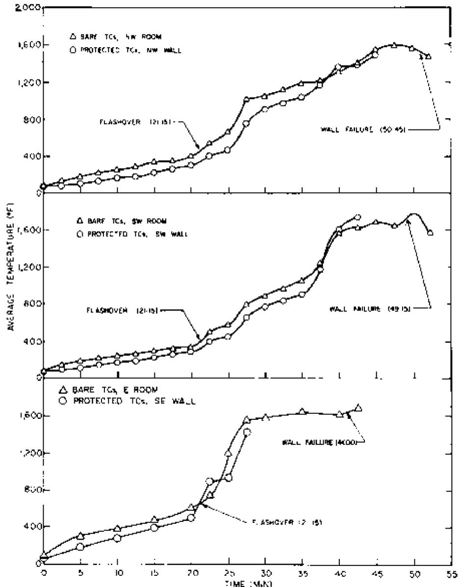
Figure 7.—Temperature development in Structure 5. (M 148 012)
