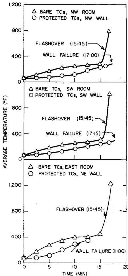
Figure 5.—Temperature development in Structure 1.
