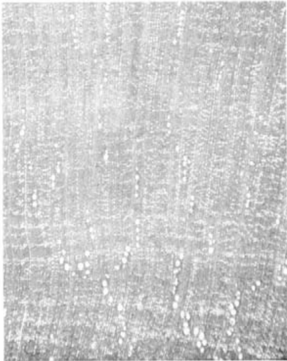
Figure 3.-- Bumelia glomerata . Compare extremes of pore size in radial-echelon arrangement. X 30.
