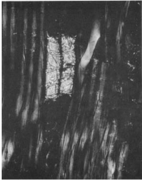
Figure 8. -- Bumelia obovata , showing two strands of two-sized crystals. Polarized light. X 275.
