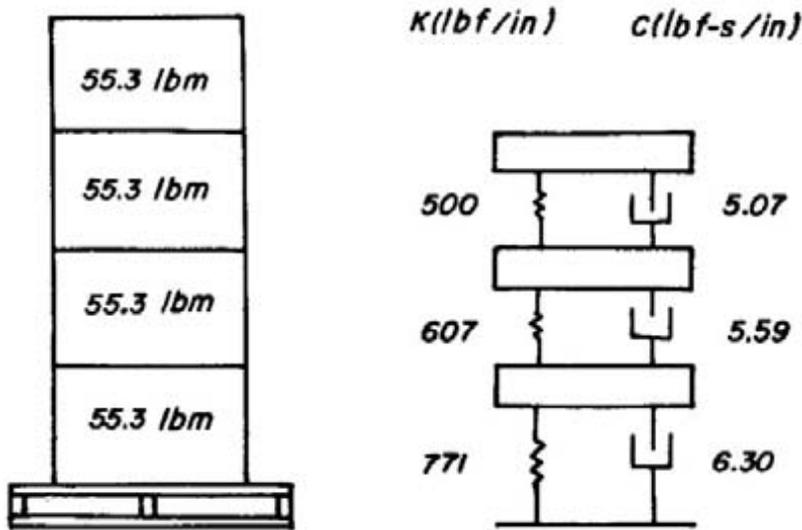
Figure 1.--Schematic diagram of a four-high stack arrangement, showing the relationship between a column of boxes and the vibration model. (M 146 029)
