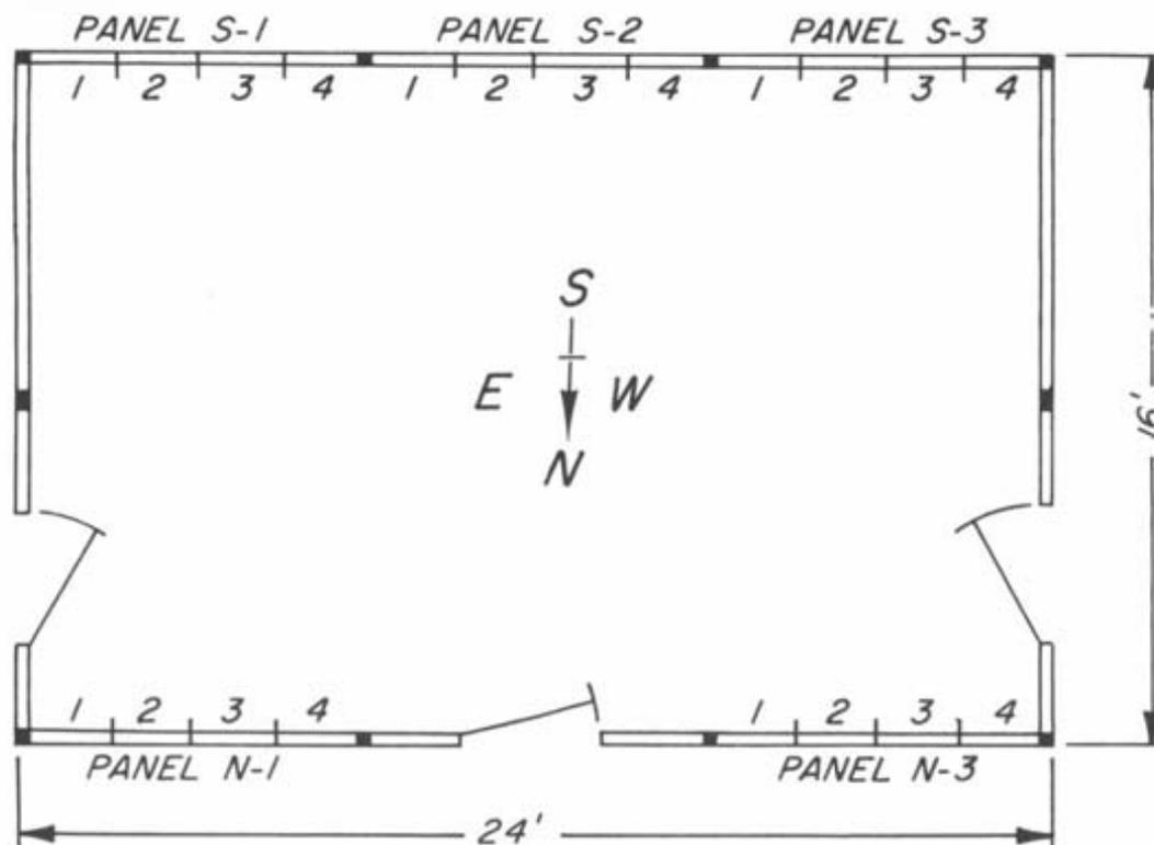
Figure 2. - - Arrangement of panels in FPL test house. (M 144897)
