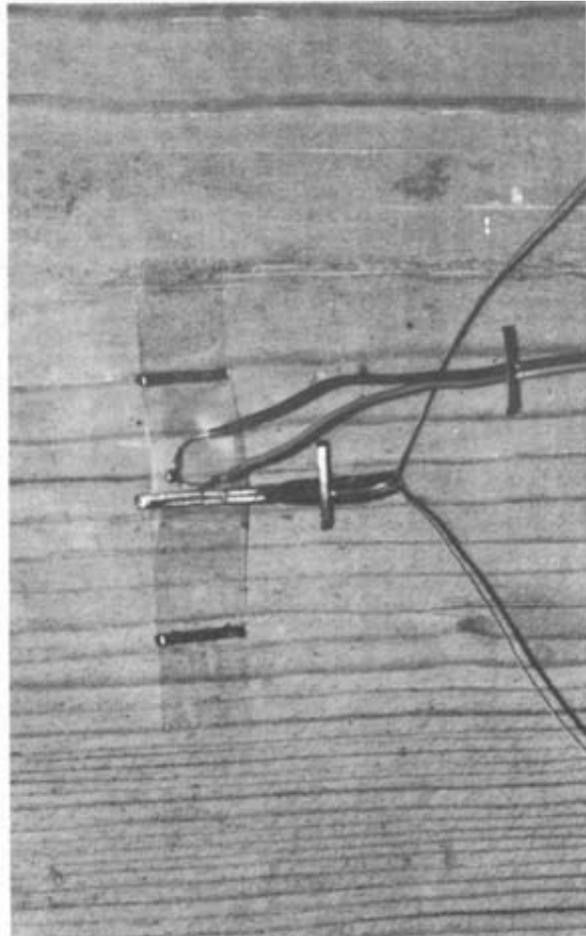
Figure 5. - - Moisture probe and thermocouple attached to interior surface of sheathing board. (M 144 309)
