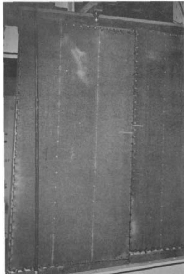
Figure 1.—Failed panel showing relative displacement and broken tension corners. (M 143 362-10)
