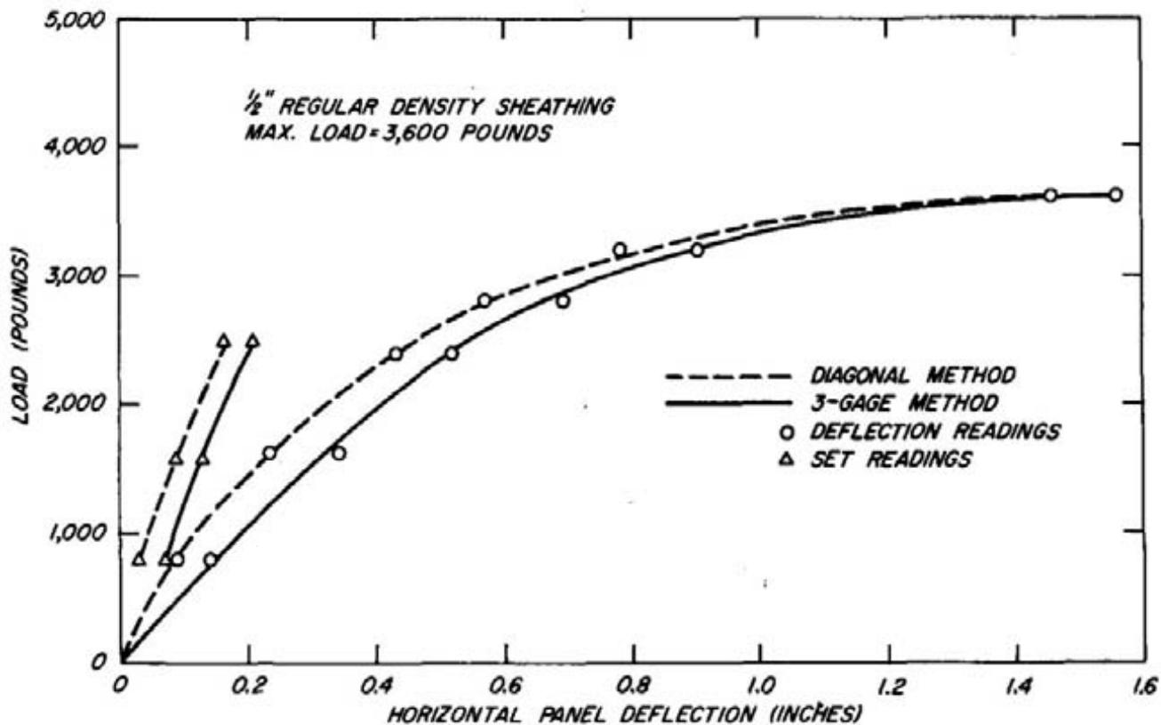
Figure 10.—Typical load-deflection curves for 8- by 8-foot panel sheathed with fiberboard by the three-gage method and diagonal displacement method.
