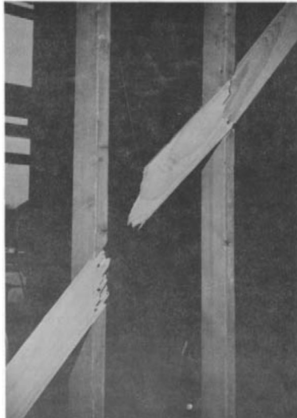
Figure 5.—Buckling failure of a type I compression brace.
