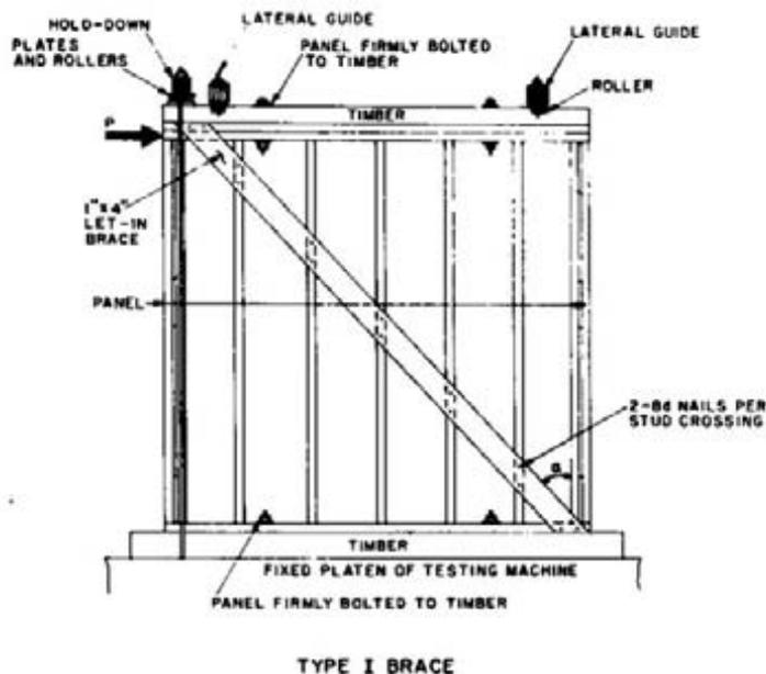
Figure 3.—Type I brace is let into the top and bottom plates and is loaded in compression. Failure is generally in a buckling mode when the brace controls ultimate strength.
