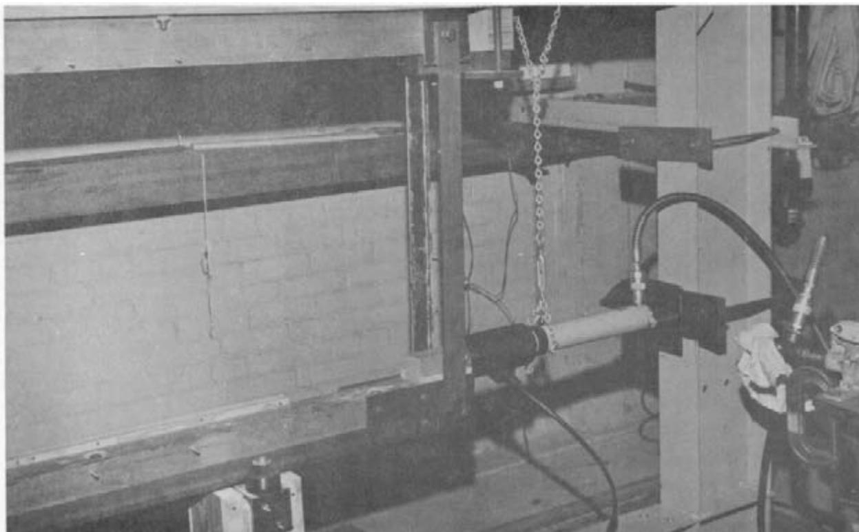
Figure 11.—Pantograph frame designed for testing small-scale racking specimens.
