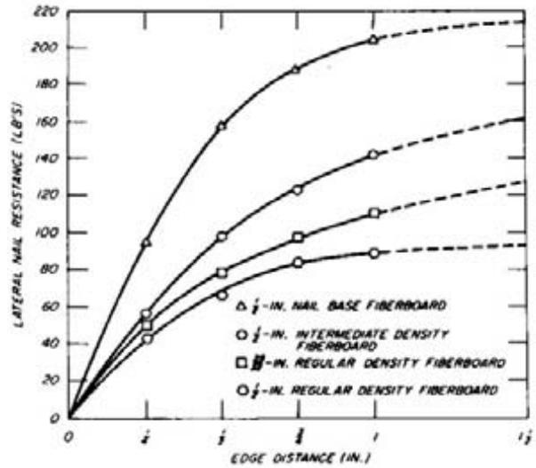
Figure 14.—Lateral nail resistance at various edge distances for four types of fiberboard shearing.
