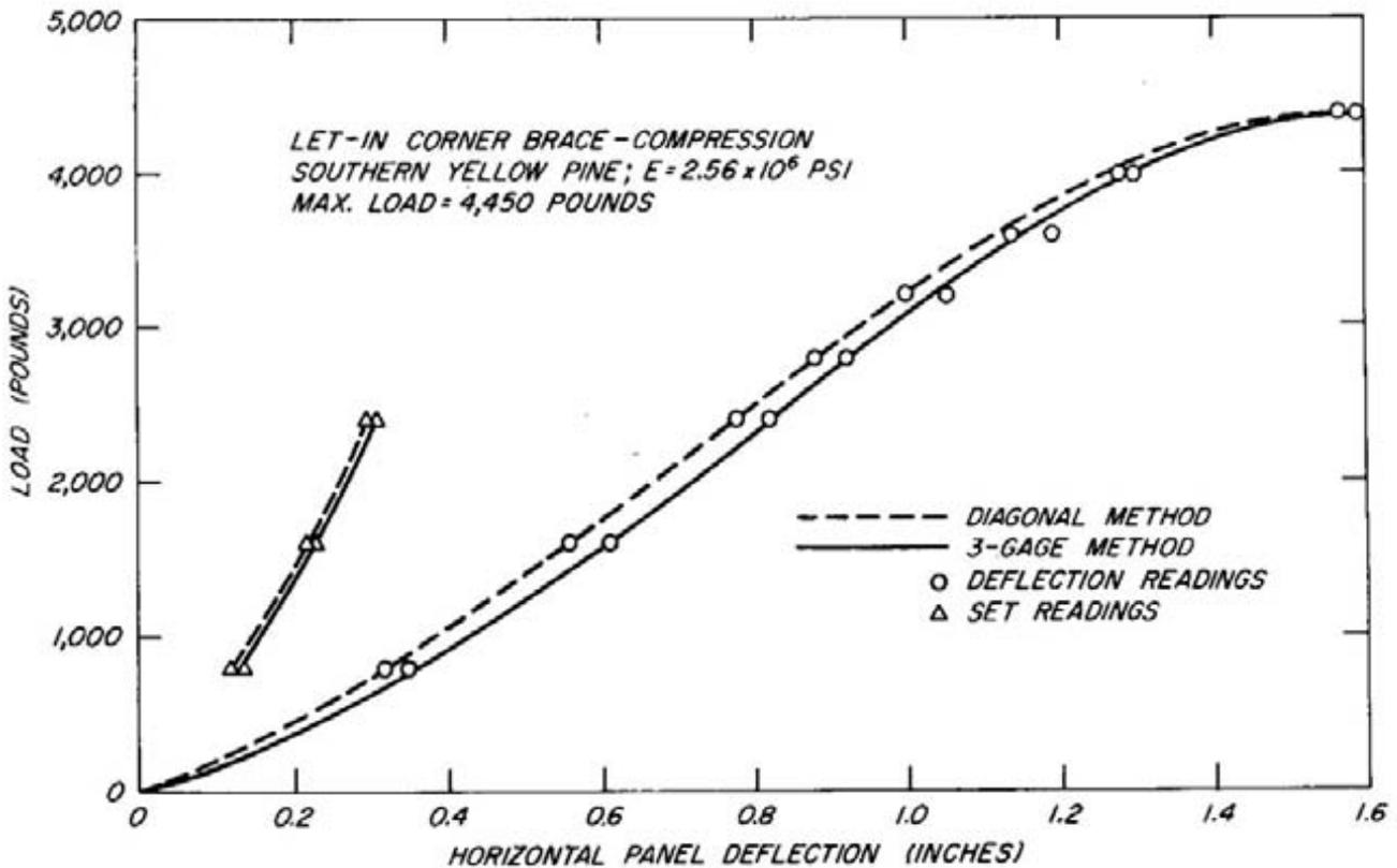
Figure 13.—Typical load-deflection curve for 8- by 8-foot panel with let-in corner brace loaded in compression. (Type 1 brace)
