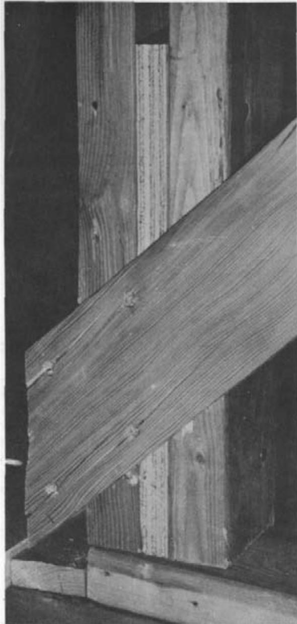
Figure 6.—Failure at the end studs of a type // brace where the load is carried by the lateral resistance of the nails.
