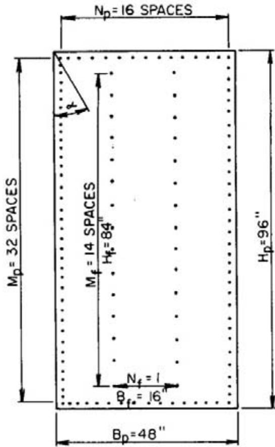
Figure 1A.—Sheet size and nail spacing for sample racking problem.
