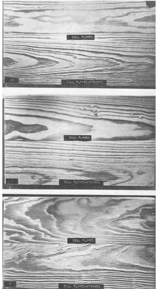
Figure 1.—Boards 4, 1, and 7 of southern pine, illustrate stress-relief (grain raising) by steaming. (M 143 621)
