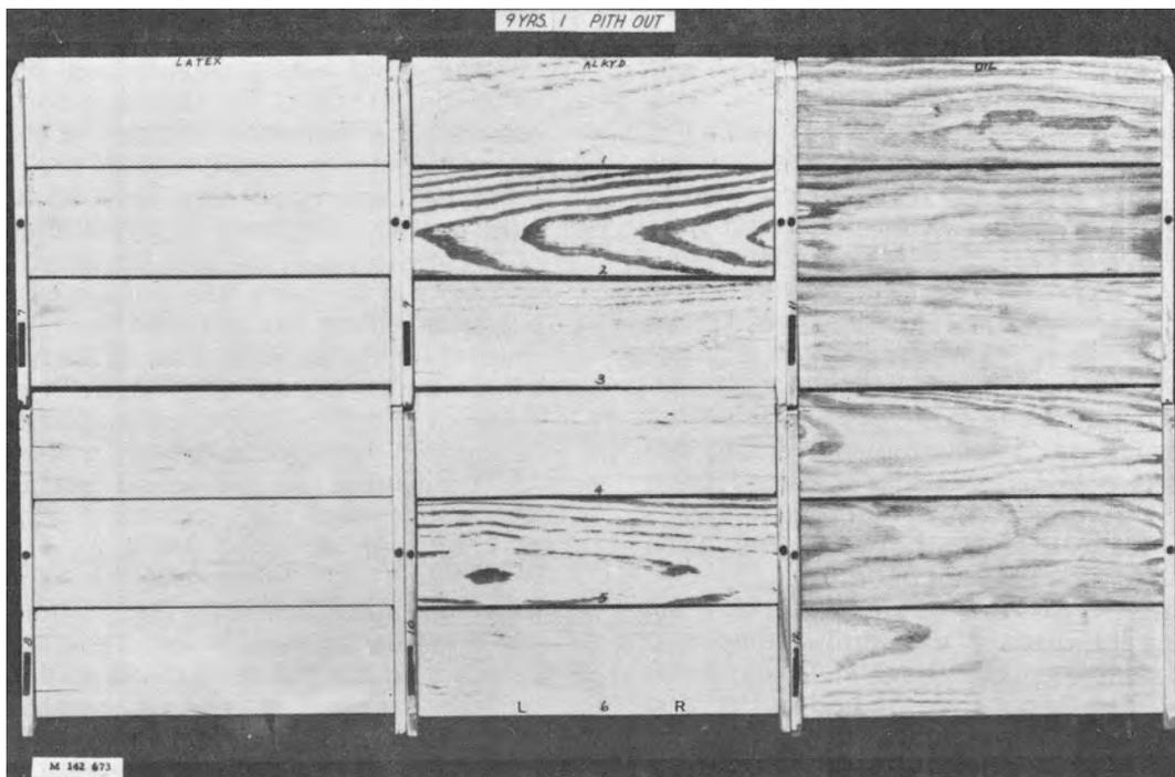
Figure 3.—Latex, alkyd, and oil-based paints after 9 years' exposure. (M 142 672)
