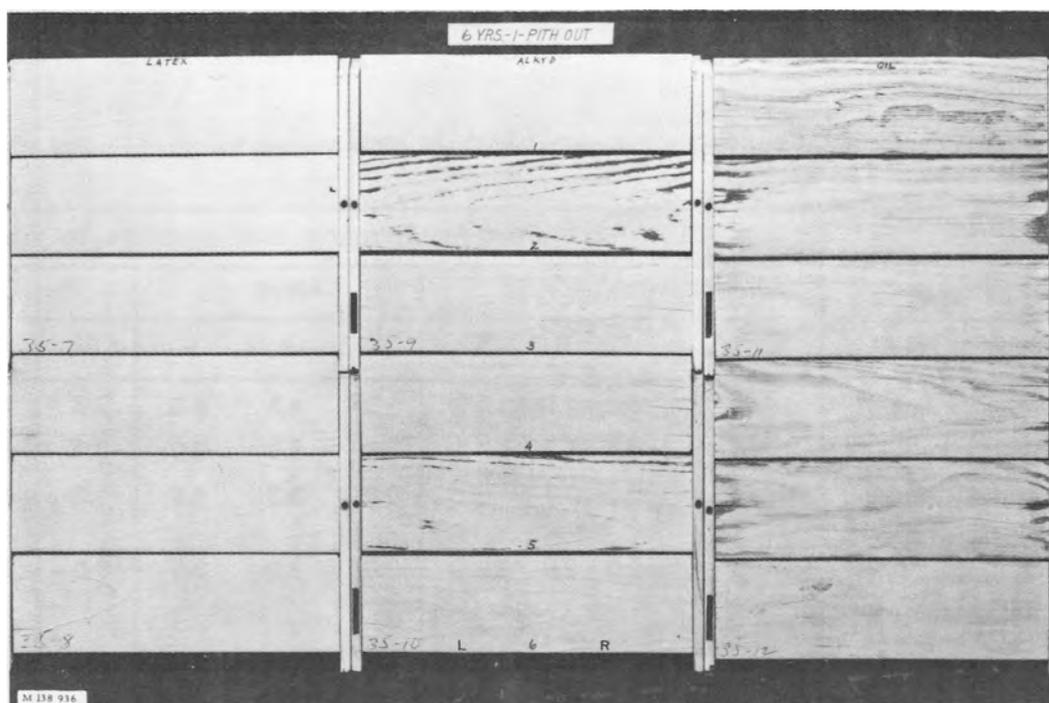
Figure 2.—Latex, alkyd, and oil-based paints after 6 years' exposure to weather. Treatment numbers are indicated on alkyd panels (first replica). Note advanced peeling failure of alkyd paint from summerwood bands on boards surfaced with sharp planer (treatment 2) and with dull planer (treatment 5). Note improved performance of oil paint over chromic acid-treated surface (treatment 6R). The performance shown here was typical of three replicas.
