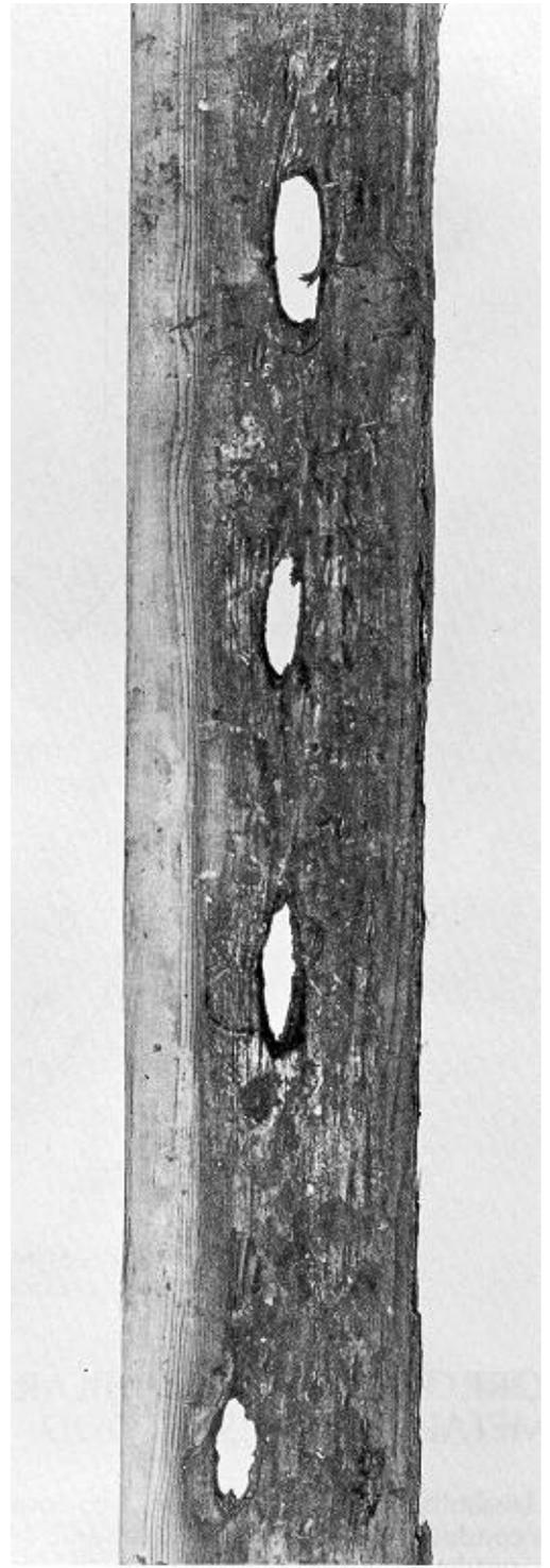
Figure 3.—Hull plank from 20-year-old wooden ship shows wood degradation around silicon bronze lag bolts. The lag bolts held a silicon bronze brace to the plank; brace and bolts were connected to ship's cathodic protection system.
