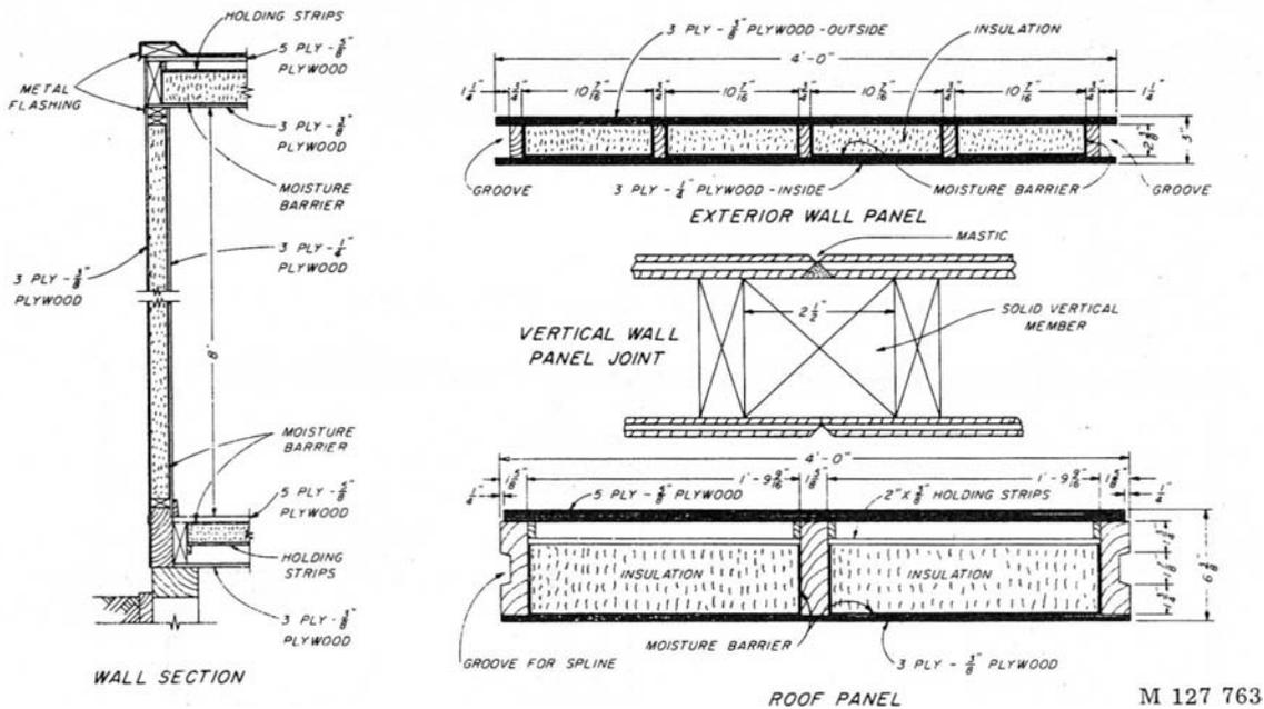
Figure 4.--Construction details of prefabricated one-story stressed-skin plywood house developed at U.S. Forest Products Laboratory, showing wall section, exterior wall panel, and roof panel.
