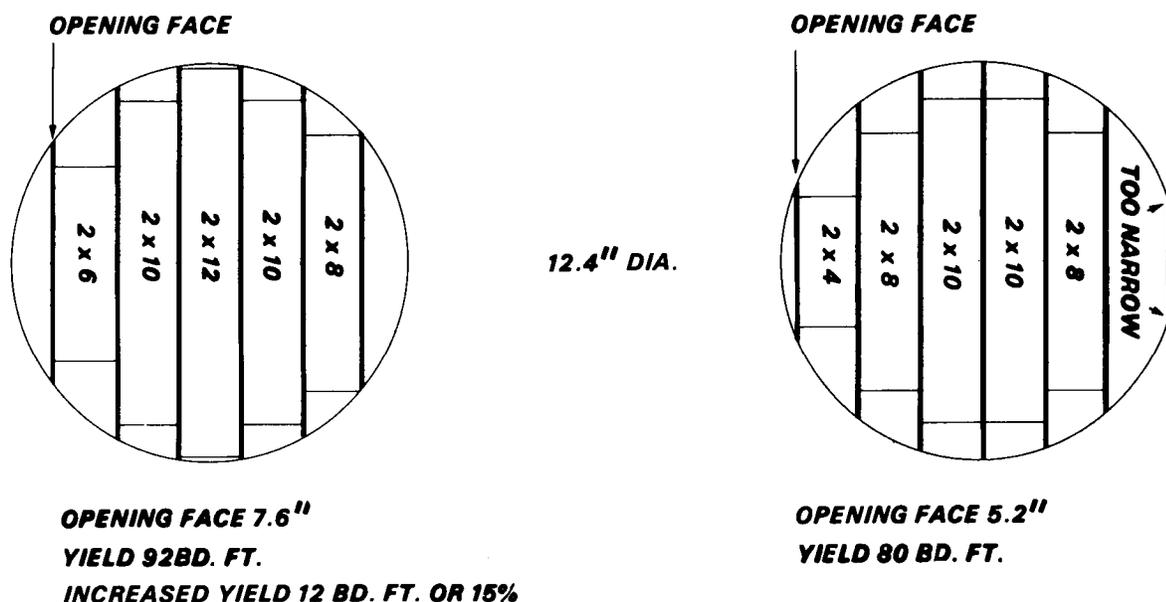
Figure 8.--The effect of two different opening faces on lumber yield for logs in the 12.4-inch-diameter class.
