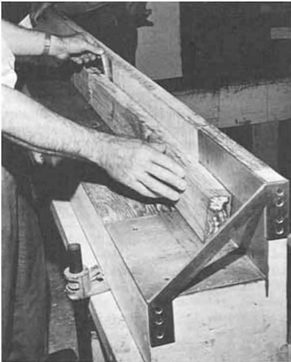
Figure 7.--Measuring crook in a stud; amount of deflection is read on a tapered wedge gage.
