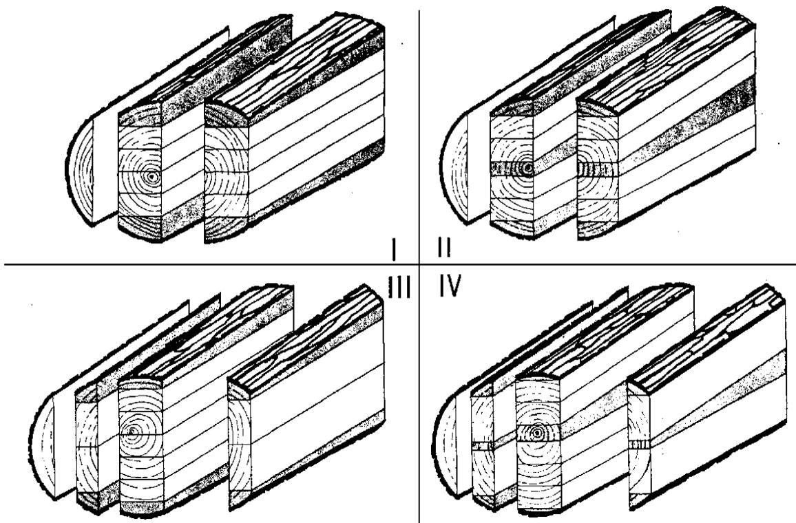
Figure 1.--Four sawing methods (on 12-inch diameter class) that can be used to reduce logs to studs. In Methods I and III taper and excess wood (shaded area) are in the slab, whereas in Methods II and IV they are mainly concentrated in a wedge in the pith area.
