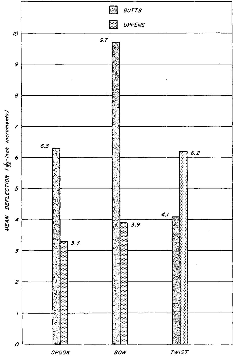
Figure 10.--Effect of log position on crook, bow, and twist for mean warp of all studs.
