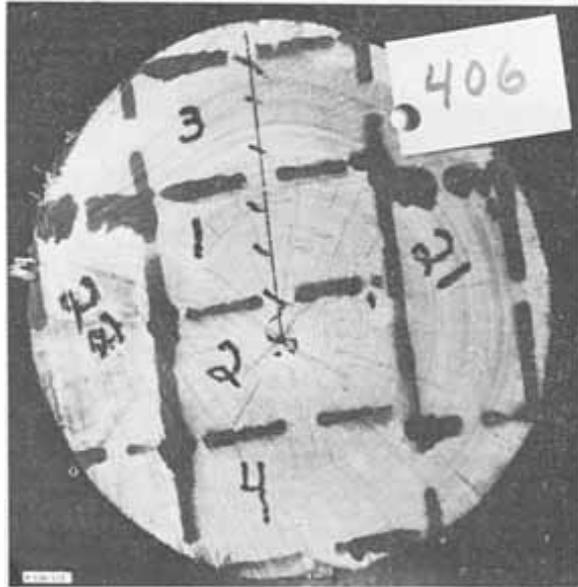
Figure 2.--Crosssection with Sawing Method III design applied to 10-inch log; cross-sectional eccentricity in vertical position. Compression wood is shown especially in studs 1 and 3.
