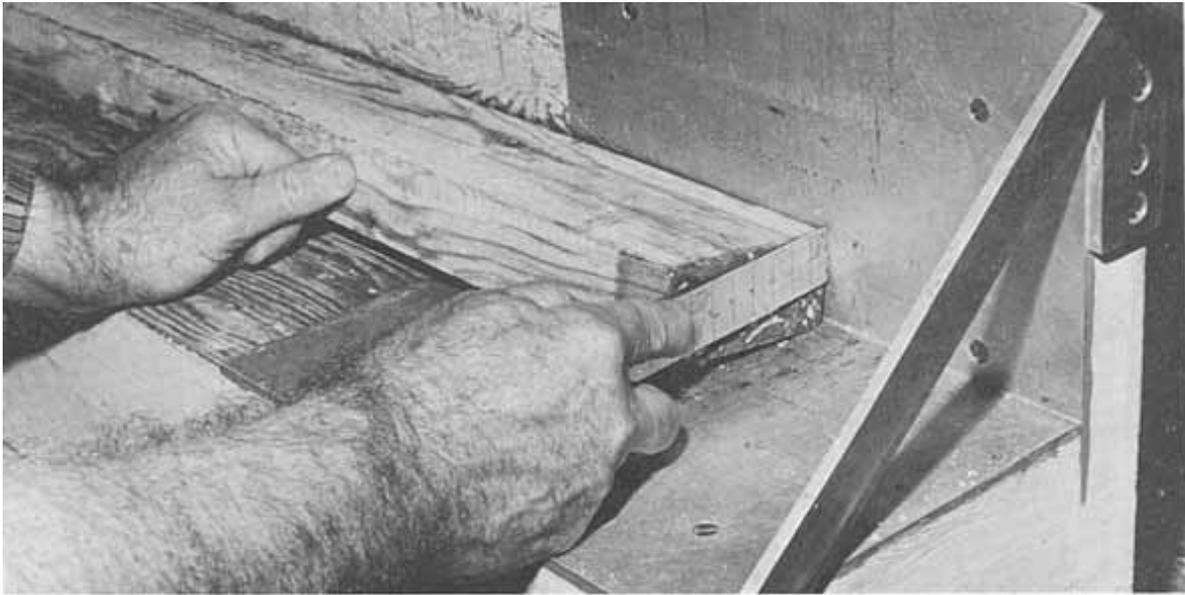
Figure 6.--Measuring the length of a stud; metal panel immediately behind stud is graduated in increments of 1/32 inch.
