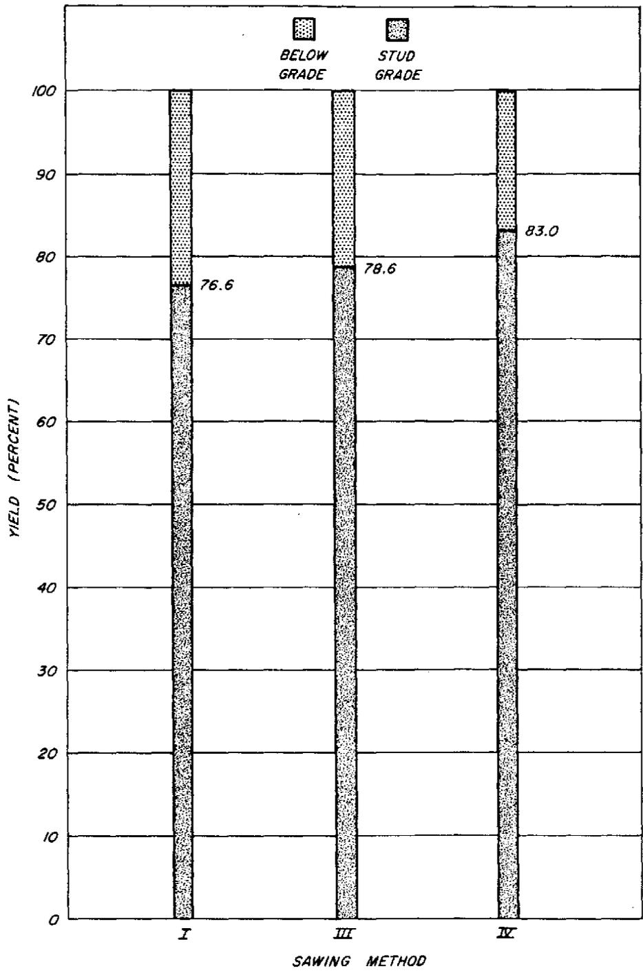
Figure 11.--Percent yields for sawing methods of studs meeting "stud" grade (National Grading Rules) from 12-inch logs (butts and uppers) in substudy 2.
