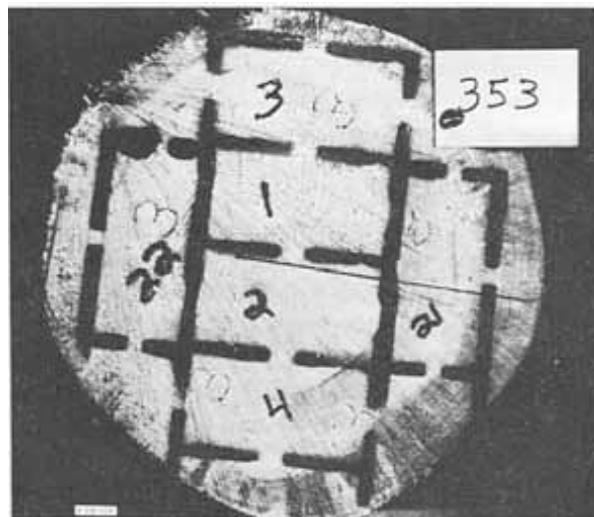
Figure 3.--Crosssection with Sawing Method III design applied to 10-inch log; cross-sectional eccentricity in horizontal position.
