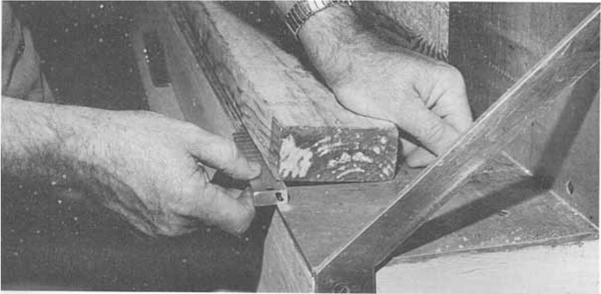
Figure 9.--Measuring twist in a stud; end of stud not shown is held flat to the table.
