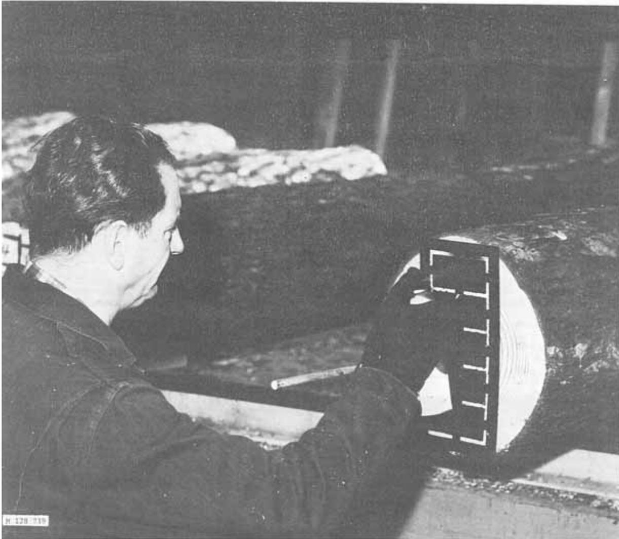
Figure 4.--Stenciling sawing pattern with an aerosol paint spray for center cant on end of log.
