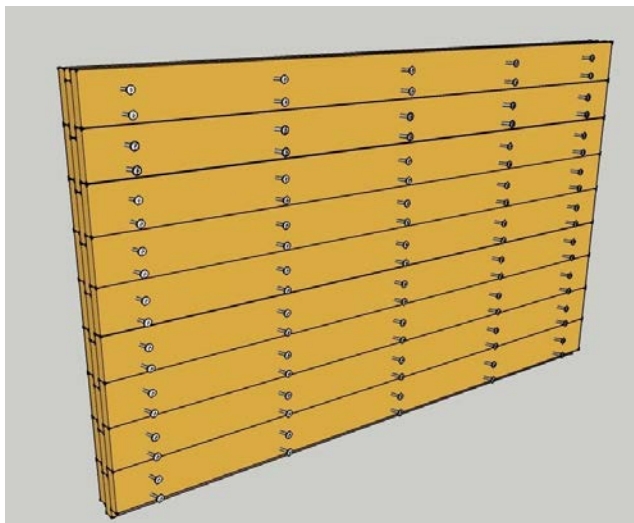
Figure 2. Assembled wall panel (without sheathing).
