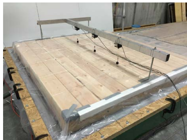
Figure 7. Ceiling panel test configuration (in this case, the plywood is on the tension side).
