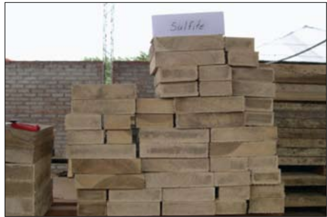
Figure 4—Cross sections of boards that were treated in sulfite solution. Note that some boards have discolored centers, others have little or no discoloration.
