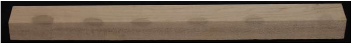
Figure 9—Hammered maple board cut open to expose extent of discoloration.
