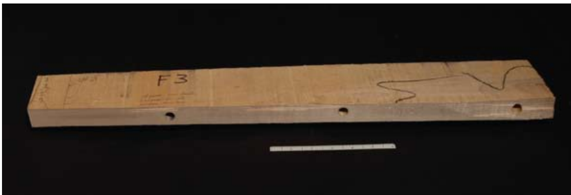
Figure 6—Board split with froe prior to clamping, storage, and drying, then edge-planed after drying to reveal depth at which discoloration begins. Note that the split surface at the right end is unstained, but that planing exposes interior stain.
