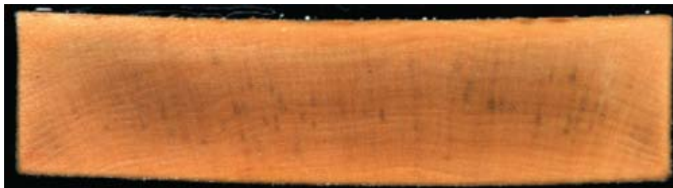
Figure 11—End-grain view showing center of board completely stained in log 2, day 5.
