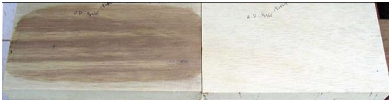
Figure 1—Ochoó boards severely affected by oxidative stain (left) and unaffected by stain (right).
