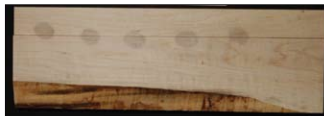
Figure 8—Surface of maple board hit with hammer, then cut open to expose extent of discoloration.
