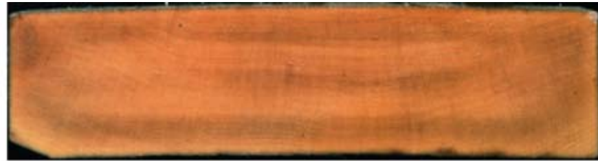
Figure 9—Hammered maple board cut open to expose extent of discoloration.
