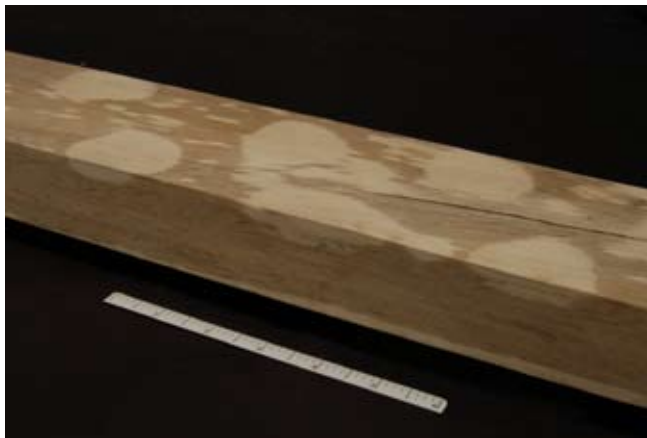
Figure 3—Surface of ochoó board hit with hammer, then cut open to expose extent of discoloration.
